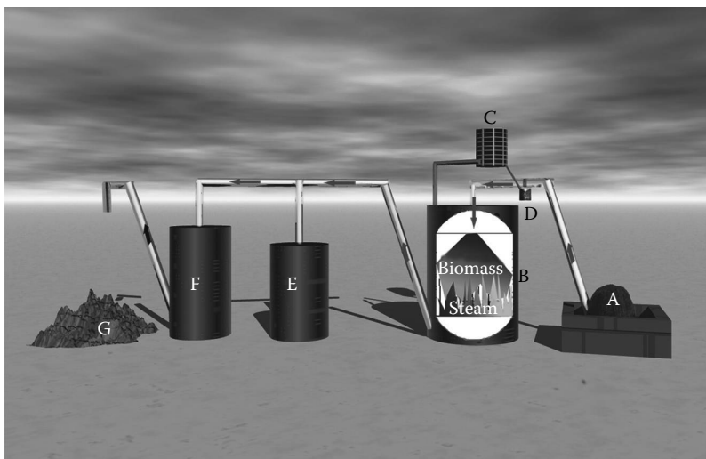
FIGURE 5.24 Scheme of the BIOLANDES continuous production unit. A, biomass; B, distillation vat; C, condenser; D, Florentine flask; E, extraction unit; F, solvent recovery; and G, exhausted biomass.
