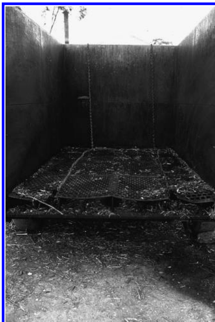
FIGURE 5.23 View inside the distillation container, showing the steam tubes and the metallic grid.
