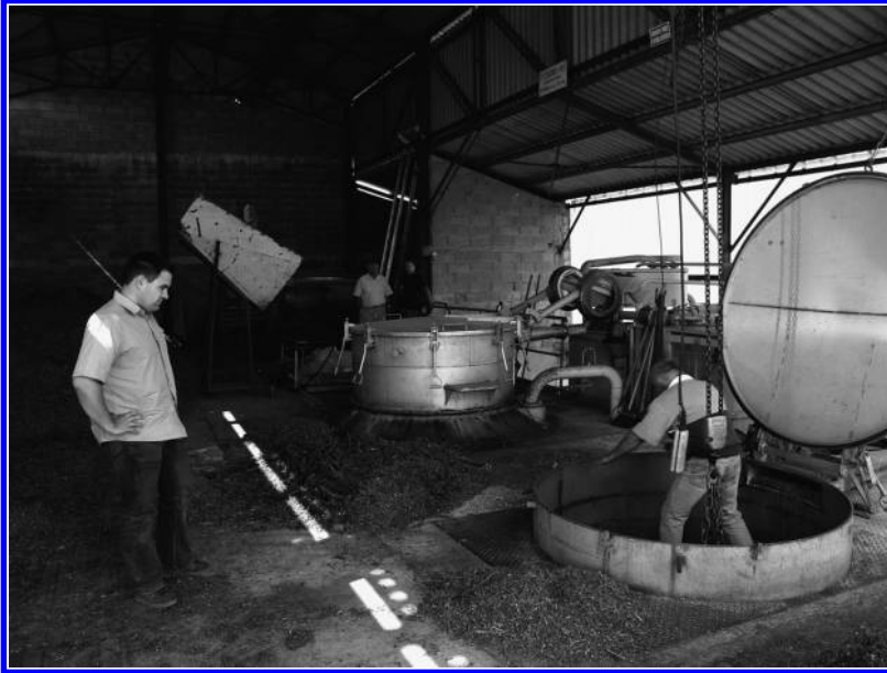
FIGURE 5.14 Loading a kettle and pressing by concreted tractor wheel.
