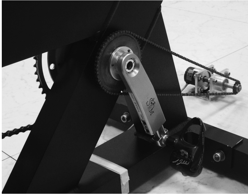
Picture 1. A rotational encoder was coupled to the left crank of the SRM ergometer in order to measure the instantaneous angular position of the crank and synchronize it with the EMG activity.
