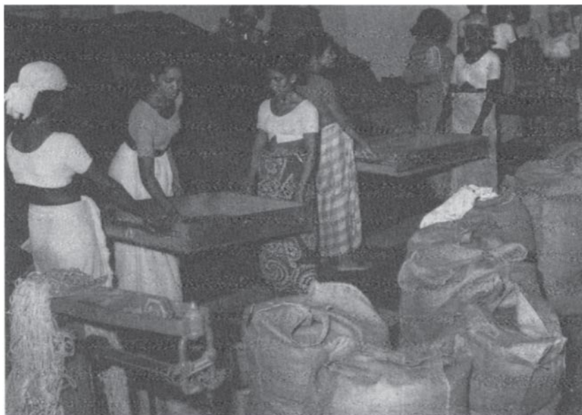
Figure 7.1.8 Garbling or grading is done manually by using sieves of specific sizes.
