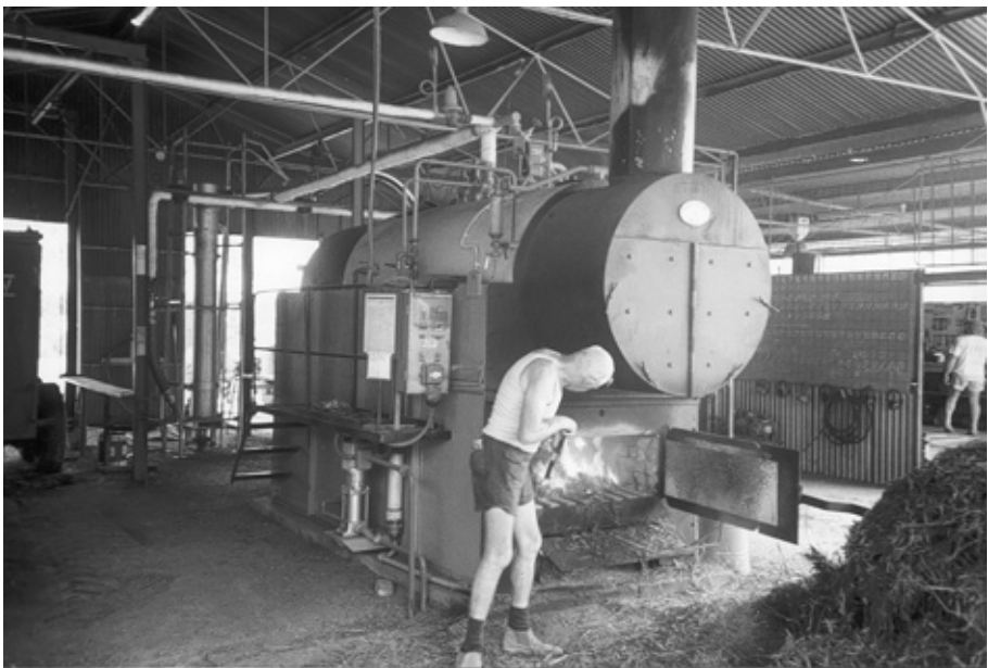
Figure 7.4 Distillery of G.R. Davis Pty Ltd showing space either side of the boiler for placement of trailer bins. Boiler uses dried spent leaf from previous distillations (photo: J. Coppen).
