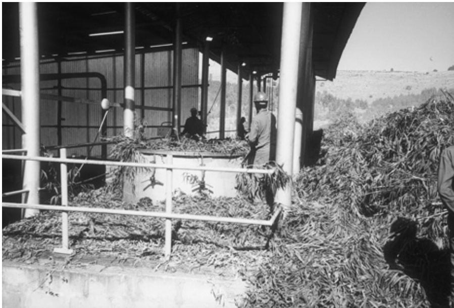
Figure 9.5 Eucalyptus smithii leaf being packed into stills for distillation, Swaziland (photo: J. Coppen).
