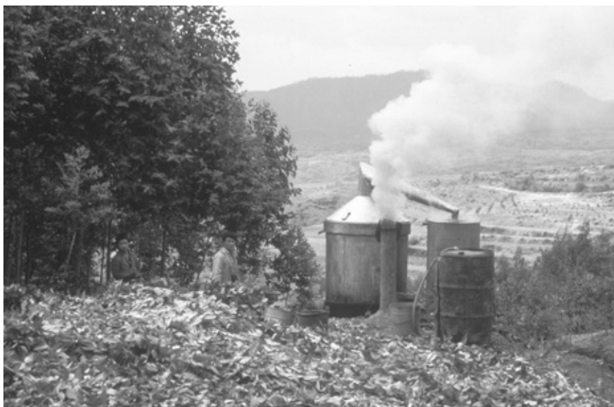
Figure 8.3 Village-scale steam distillation of Eucalyptus globulus , near Chu Xiang City, Yunnan Province (photo: S. Midgley).
