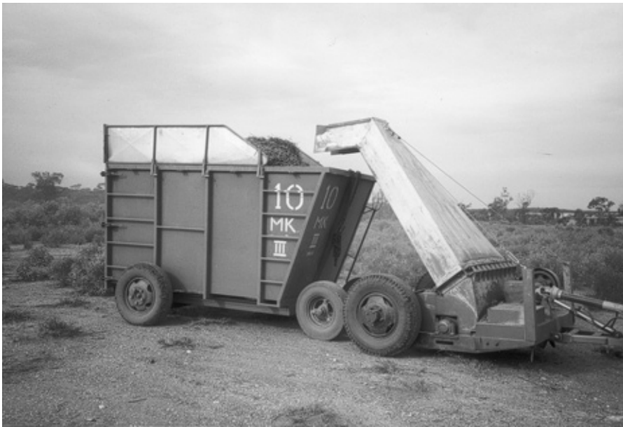
Figure 7.2 Trailer bin, which also functions as a still, packed during mechanical harvesting of Eucalyptus polybractea , West Wyalong, New South Wales (photo: J. Coppen, courtesy of G.R. Davis Pty Ltd).
