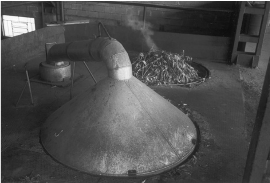
Figure 10.3 Pair of stills sharing a single lid and condenser (photo: J. Coppen).
