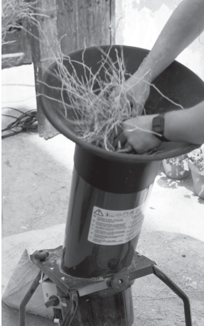
Figure 3.13 It is possible to use normal shredders for wood or plant material to cut the roots in small pieces before distillation.
