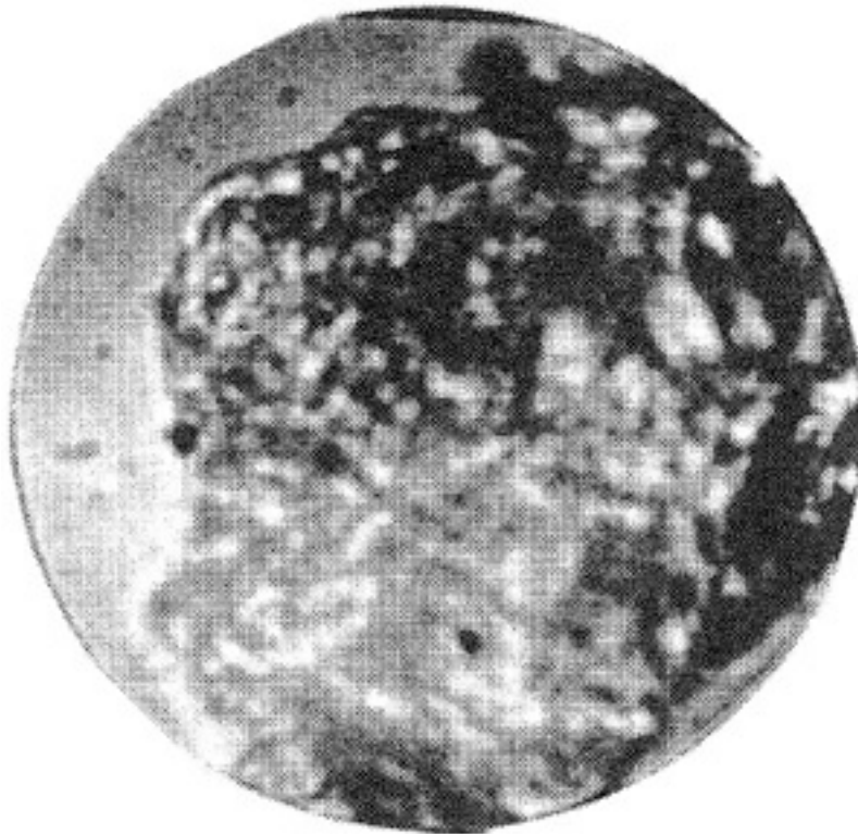
Figure 33. Crystal in early stages of vesicular structuring. Preparation 1a, six weeks old. 1000x
