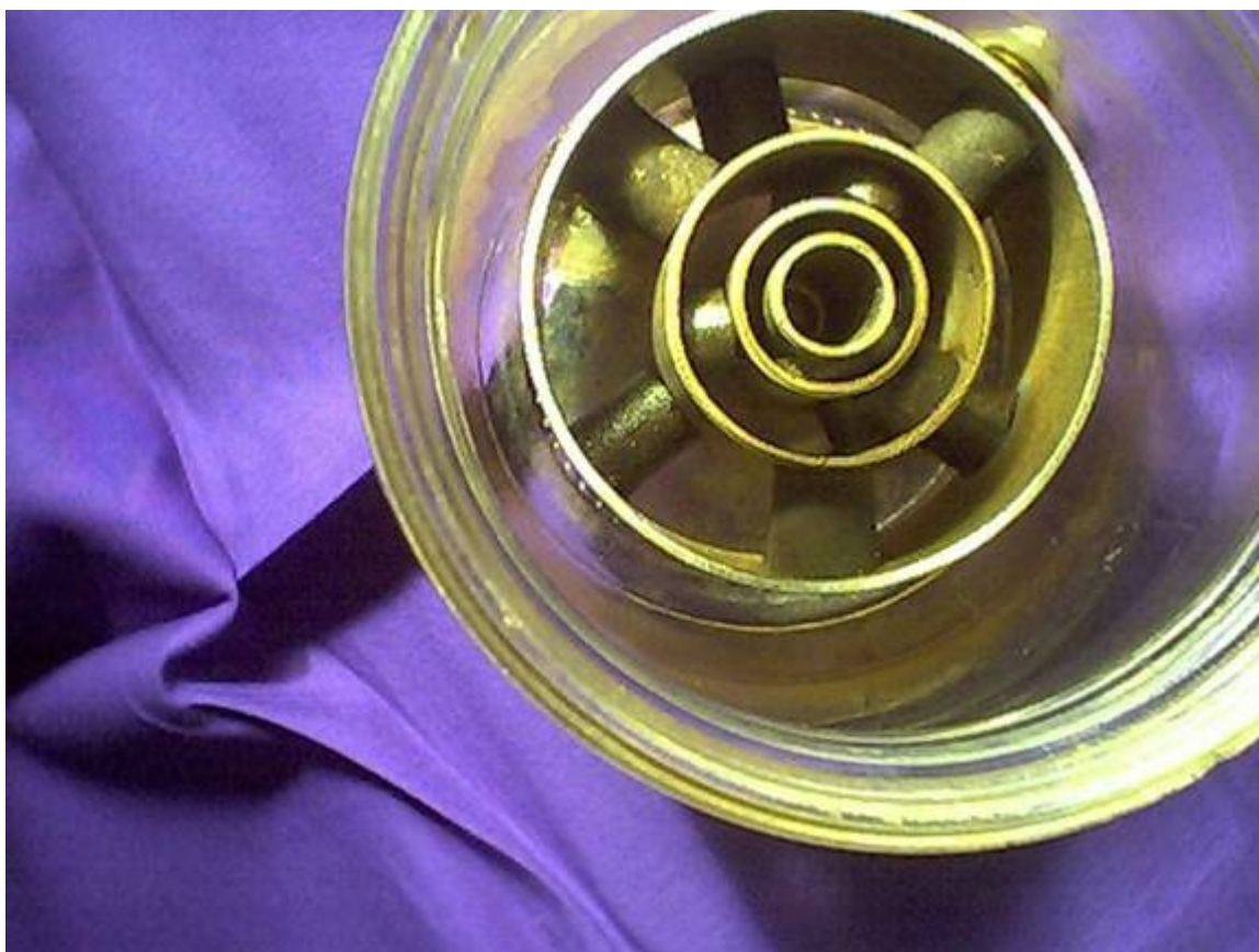
Figure showing radial arrangement of spacers.
