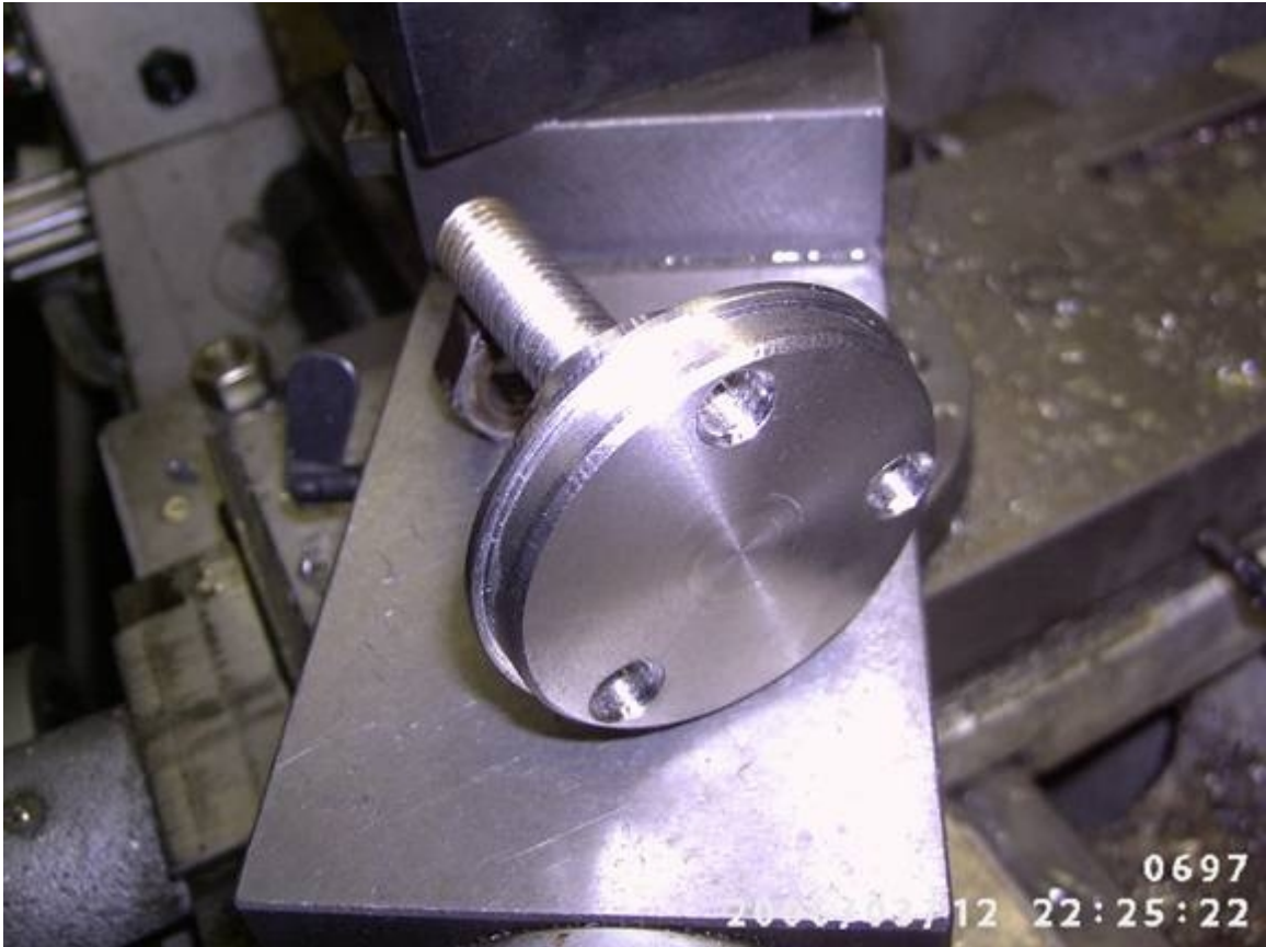
Figure showing hub from the top. Observe the penetrating holes to permit water flow.
