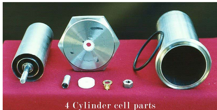
Fig.16B — Pile, 4 cylindres.
