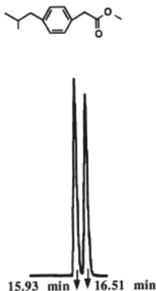
Figure 6.15 The Separation of the Enantiomers of Ibuprofen Courtesy of ASTEC Inc.
