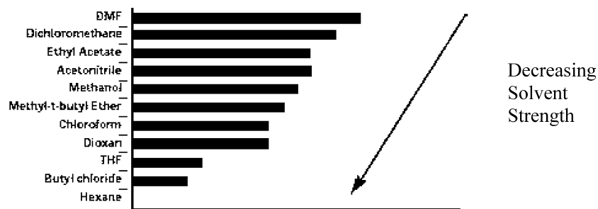
Fig. 3 Solvent strength data on porous graphitized carbon columns for the retention of aniline, naphthalene, ethyl benzene, and phenol. (Reproduced by kind permission of Thermo-Hypersil-Keystone.)
