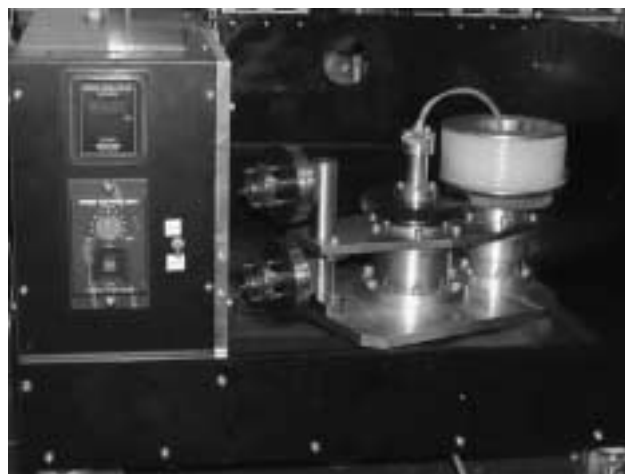
Fig. 1 Photograph of the type-J multilayer coil planet centrifuge. (View this art in color at www.dekker.com .)
