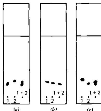
Figure 9.13 TLC separations of 1,7-dimethoxynaphthalene (1) and 1-nitronaphthalene (2) on silica plates; (a) 20%v benzene/pentane solvent, (b) 1%v acetonitrile/pentane solvent (no presaturation), (c) 1%v acetonitrile/pentane solvent (10-min presaturation). Reprinted from (7) with permission.
