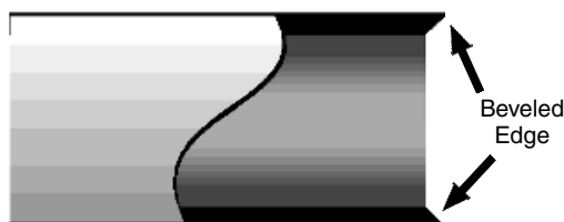
FIGURE 10.16 Trim and bevel a newly cut tubing end [reprinted with permission of Supelco, Bellefonte, PA 16823 (USA)].
