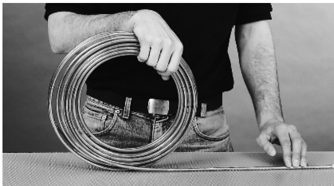
FIGURE 10.15 Uncoil tubing without creating bends [reprinted with permission of Supelco, Bellefonte, PA 16823 (USA)].
