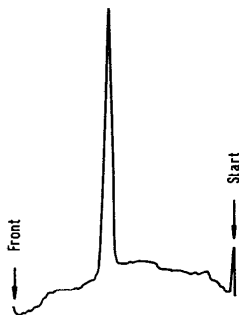
Fig. 1: Reflectance scan of a chromatogram of 200 ng D- \alpha -tocopherol per chromatogram zone.
