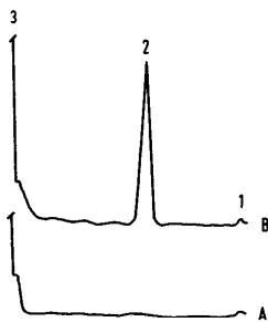
Fig. 1: Fluorescence scan of (A) a blank and (B) a carbamazepine standard with 200 ng per chromatogram zone. Start (1), carbamazepine (2), solvent front (3).
