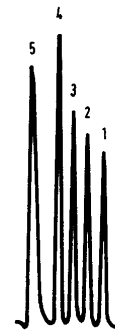
Fig. 2: Fluorescence scan of a \Delta^4 -3-ketosteroid mixture after INH treatment. Aldosterone (1), corticosterone (2), cortexolone (3), testosterone (4), progesterone (5).
