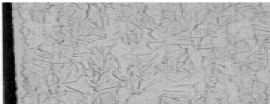
Plate 2 Backscattered electron image of a cross-section of a nitrided low alloy steel (left) and quantitative rf-GD-OES depth profile of 'ionic' nitrided low alloy steel.
