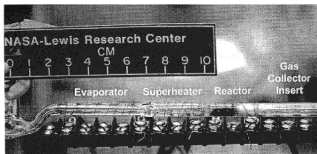
Figure 5. Miniature reformer showing the evaporator, superheater, reactor, and gas collection insert. The catalyst in the picture is in powder form. 37
