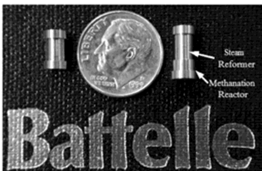
Figure 2. Battelle subwatt power microreformers. (Reprinted with permission from ref 41. Copyright 2002 Elsevier.)
