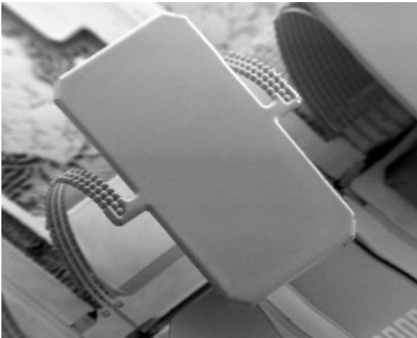
Fig. 10.10 SEM micrograph of a tunable IR Bragg filter ( 1.1 \times 1.85 mm) of density-modulated PS, suspended at two microactuator arms. Its rest position is more than 180^\circ
