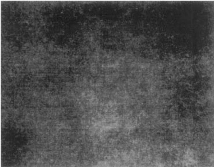
Figure 16: Normarski micrograph of a diamond turned copper surface before recrystallization (100 \times ). From reference 42. Reprinted with permission of the American Electroplaters & Surface Finishers Soc.
