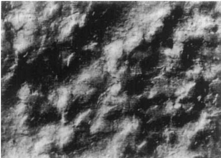
Figure 17: Normarski micrograph of a diamond turned copper surface after recrystallization (100 \times ). From reference 42. Reprinted with permission of the American Electroplaters & Surface Finishers Soc.
