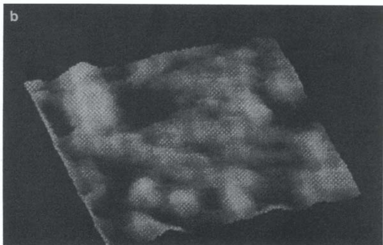
Figure 10. (A, B, C) AFM images of an aluminum surface corroding in seawater. The images were taken approximately 1 1/2 min apart. The scan area was 450 \times 450 nm. Further microscope development is being focused on lowering the drift so that processes can be observed over smaller scan areas for times of up to an hour. (Reprinted from Ref. 30 by permission of Kluwer Academic Publishers.)
