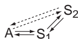
Figure 8 Illustration of single scattering (dashed line) and multiple scattering (solid lines) pathways. The absorbing atom is A, which is surrounded in this example by two scattering atoms, S_1 and S_2 .
