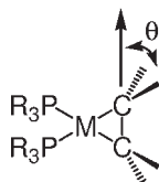
Figure 7.1 Coordination of an olefin to the transition metal fragment M(PPh_3)_2 ( M = \text{e.g. Ni, Pd, Pt} ) leads to a deviation from planarity of the olefin system. The angle \theta is a measure of the deformation of the groups attached to the carbon–carbon double bonds from planarity.
