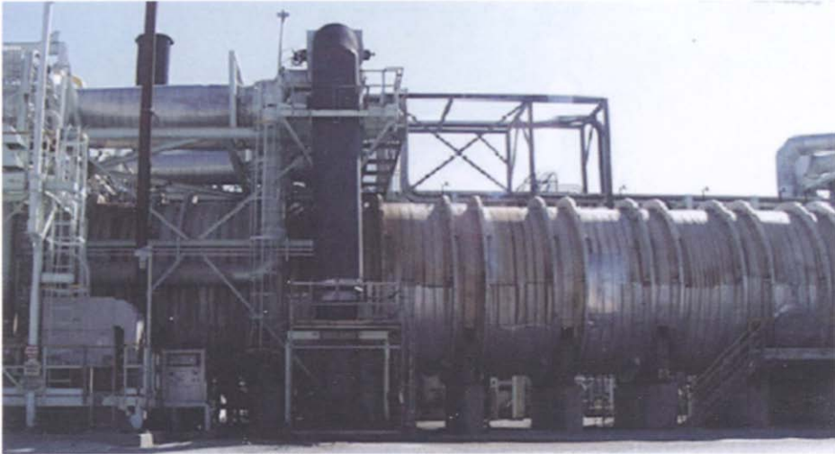
Fig. 5.2. Spent acid decomposition furnace. It is brick lined steel ~4 m diameter and 20 m long. The energy for decomposing \text{H}_2\text{SO}_4(\ell) into \text{SO}_2(\text{g}) , \text{O}_2(\text{g}) and \text{H}_2\text{O}(\text{g}) and for evaporating water is provided by burning molten sulfur and natural gas with hot air. Industrial details are given in Table 5.2.
