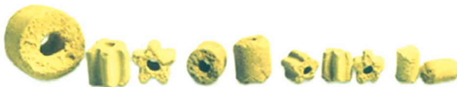
Fig. 8.1. Photograph of catalyst pieces, courtesy Haldor Topsoe A/S www.haldortopsoe.com . Rings, daisy (star) rings and pellets are shown. The daisy rings maximize catalyst area and minimize resistance to gas flow. In operation (700-900 K), the catalyst consists of a molten vanadium-alkali metal sulfate/pyrosulfate layer on a porous solid silica substrate. The outside diameter of the largest piece (far left) is 20 mm.
