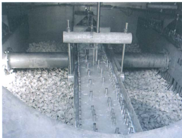
Fig. 1.3. Top of H 2 SO 4 -making ('absorption') tower, courtesy Monsanto Enviro-Chem Systems, Inc. www.enviro-chem.com The tower is packed with ceramic saddles. 98.5 mass% H 2 SO 4 , 1.5 mass% H 2 O sulfuric acid is distributed uniformly across this packed bed . Distributor headers and 'downcomer' pipes are shown. The acid flows through slots in the downcomers down across the bed (see buried downcomers below the right distributor). It descends around the saddles while SO 3 -rich gas ascends, giving excellent gas-liquid contact. The result is efficient H 2 SO 4 production by Reaction (1.2). A tower is ~7 m diameter. Its packed bed is ~4 m deep. About 25 m 3 of acid descends per minute while 3000 Nm 3 of gas ascends per minute.
