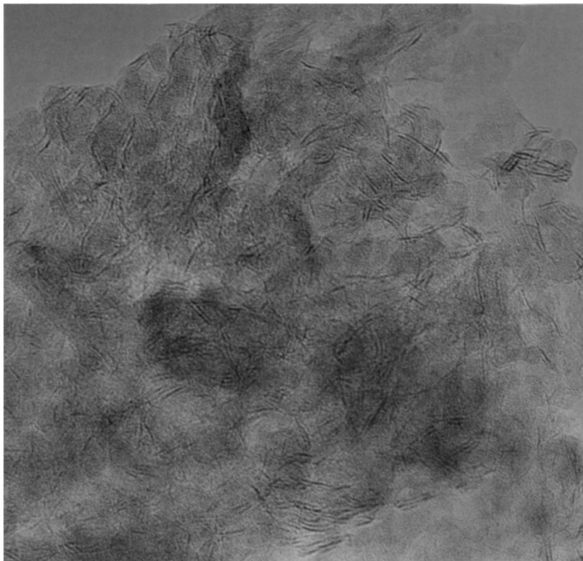
FIG. 2. TEM image of a sulfided Ni-Mo/Al 2 O 3 catalyst.
