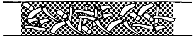
Figure 9. Testing of full sized catalyst particles by dilution with small inerts (adapted from Ref. 23).
