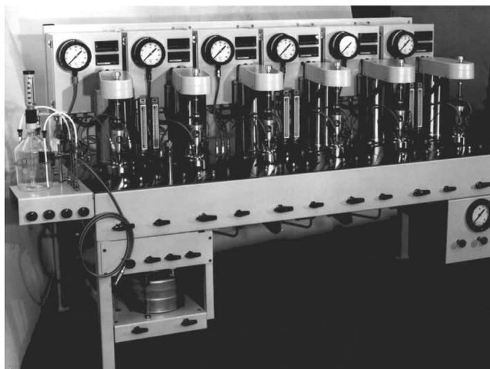
**Figure 11.31** Photograph of a sixfold autoclave bench developed by Parr Instrument Company ([www.parrinst.com](http://www.parrinst.com)). The apparatus was built in 1988, similar technologies that Parr commercialized in the early 1990s were already fully computer controlled.
