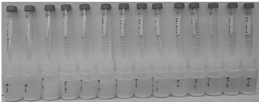
**Figure 6.21** A typical adsorption experiment, in this case for CPA on alumina. The alumina powder has been allowed to settle and is visible at the bottom of each bottle. Filtered solutions for ICP analysis are placed in test tubes.
