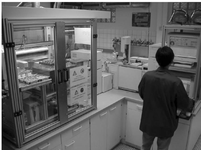
**Figure 11.35** Image of the integrated Stage I screening system employed for liquid-phase catalysis.
