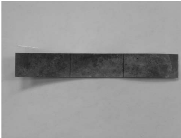
Figure 10.2. IPMC with three segment design
