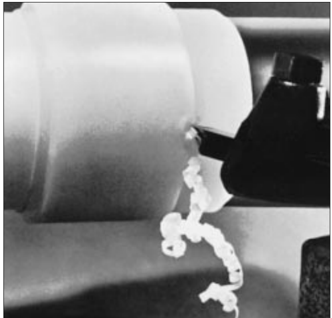
Fig. 11.04 Turning Machining conditions: Lathe speed, 980 rpm; cutting speed 185 m/min; feed 0,15 mm; depth of cut, 2,5 mm; No coolant. Material – ZYTEL® E101 – 60 mm diameter.
