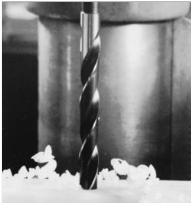
Fig. 11.03 Drilling Machining conditions: Drill size, 10 mm; Speed 1000 rpm; No coolant. Material – ZYTEL® E101 – 35 mm thick.
