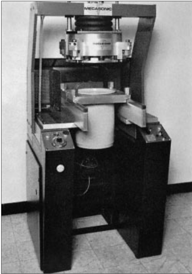
Commercial linear and angular welding machine. Manufacturer: Mecasonic SA, Zone industrielle, Rue de Foran, Ville-la-Grand, Case postale 218, 74104 Annemasse Cédex, France.
