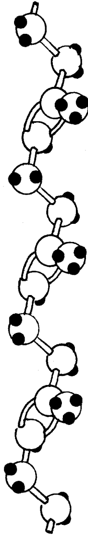
Figure 10.3. Ball-and-stick model of gutta-percha ( trans -1,4-polyisoprene).
