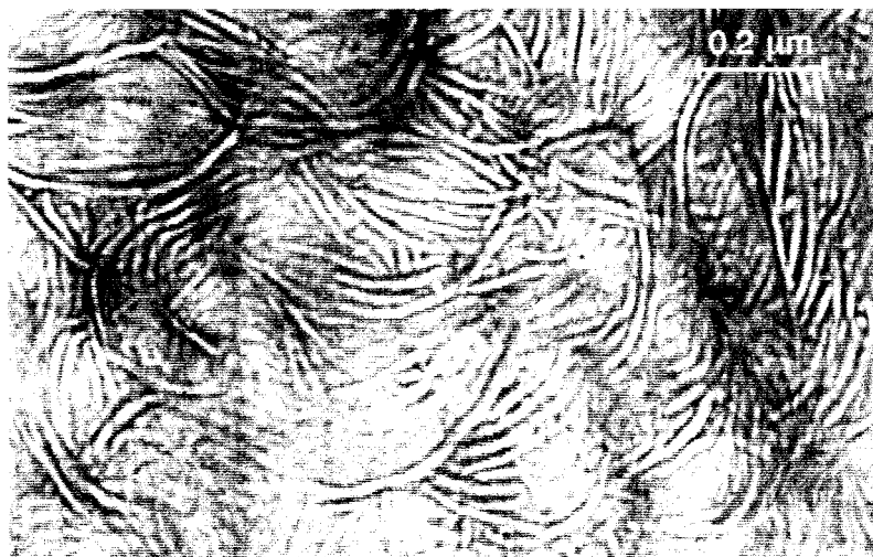
Figure 13 Partially ordered lamellar arrays in a low molecular weight ( M_w \approx 46,000 ) fraction of high density polyethylene quench-crystallized from the melt. (From Ref. 98.)
