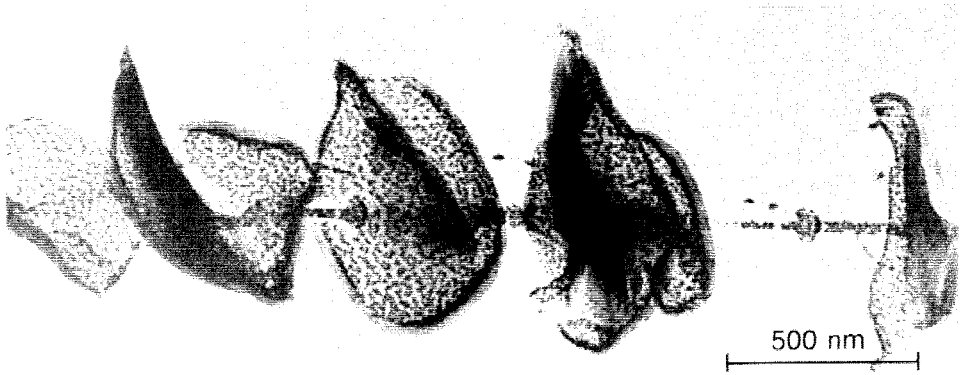
Figure 36 Electron micrograph of “shish kebab” structure grown from a stirred dilute solution of ultrahigh molecular weight polyethylene in xylene. (From Ref. 108.)
