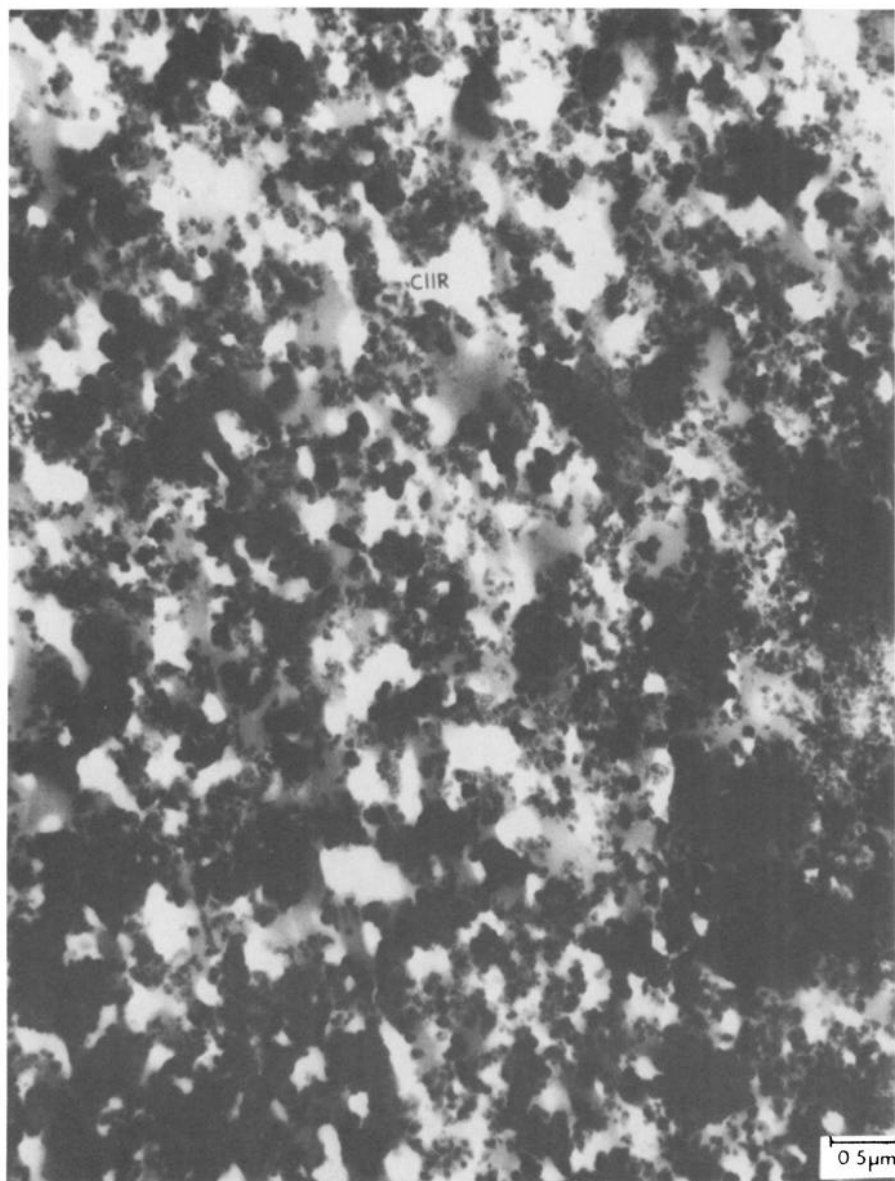
Figure 13. Location of carbon black in a blend of chlorobutyl and natural rubber & EPDM.
