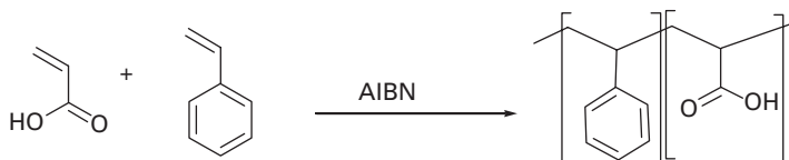
Scheme 7 A copolymer formed from styrene and acrylic acid.
