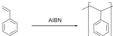
Scheme 5 Polymerization of styrene initiated by AIBN.
