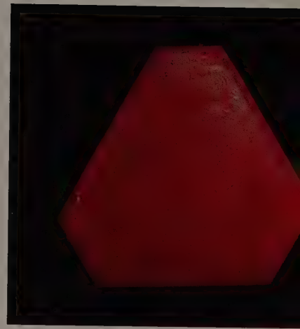
This crystal of ruby was grown hydrothermally by the Airtron Corporation.
