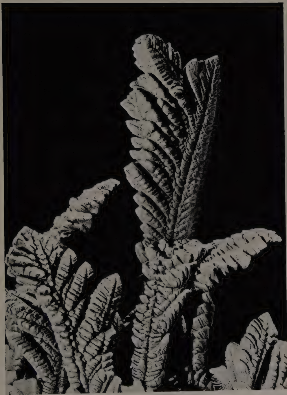
Magnesium crystals, produced accidentally in smelters, sometimes grow as dendrites.
