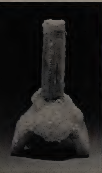
Sapphire (aluminum oxide) is rarely grown from a vapor. This crystal is less than an inch long.
