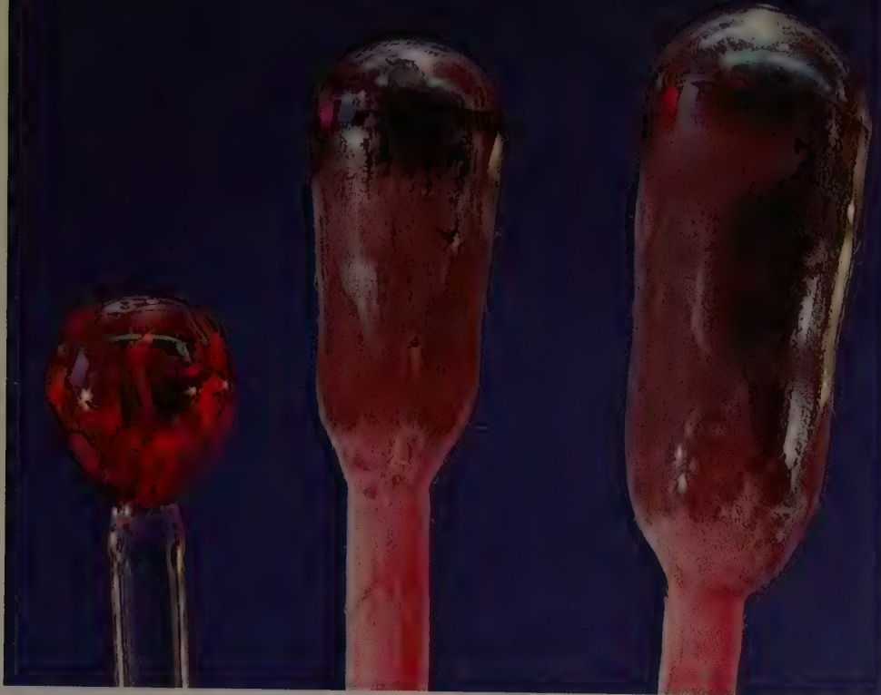
These boules (ruby) were grown by the Verneuil method. Crystals up to 9 inches in length can be produced routinely.
