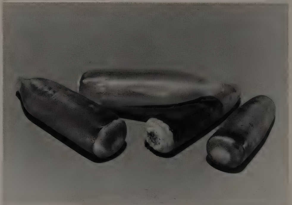
Large disc boules of ruby are grown by allowing the molten droplets in a Verneuil furnace to fall onto the edge of a rotating disc. Large round "windows" of ruby can be obtained by slicing out the centers of such boules.
