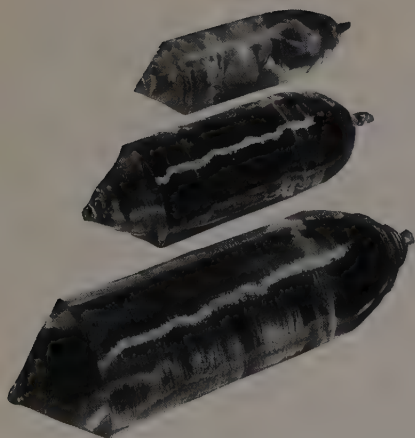
Crystals of colorless corundum (sapphire) of enormous size are routinely grown by the Czochralski method.
