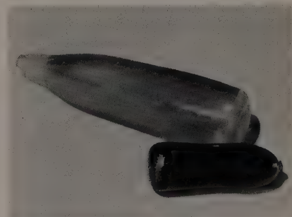
Gem-quality spinel crystals of many hues are grown by the Verneuil method.
