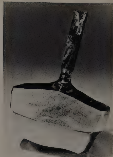
Germanium crystals are purified by zone refining in “boat-shaped” containers. The resulting material has very few impurities.
