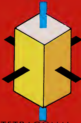
TETRAGONAL All axial angles 90 degrees, 1 axis unique.
