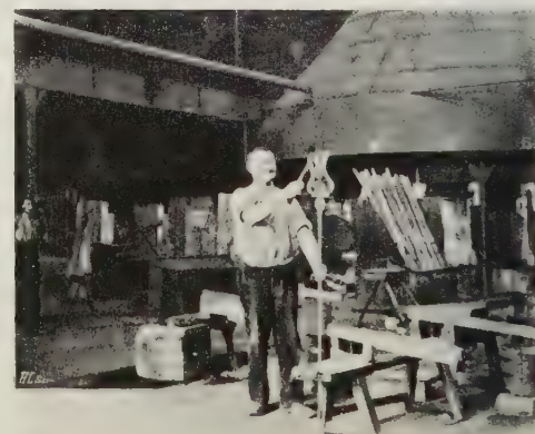
Gaffer putting the finishing touches to a glass vase still fixed to the punty, c1910. (Contemporary photograph)
