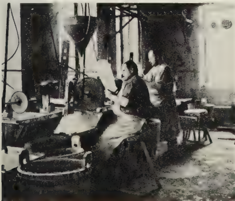
Decorator carving a vase using a wheel operated by a treadle at the Baccarat glassworks, c1910. (Contemporary photograph)
