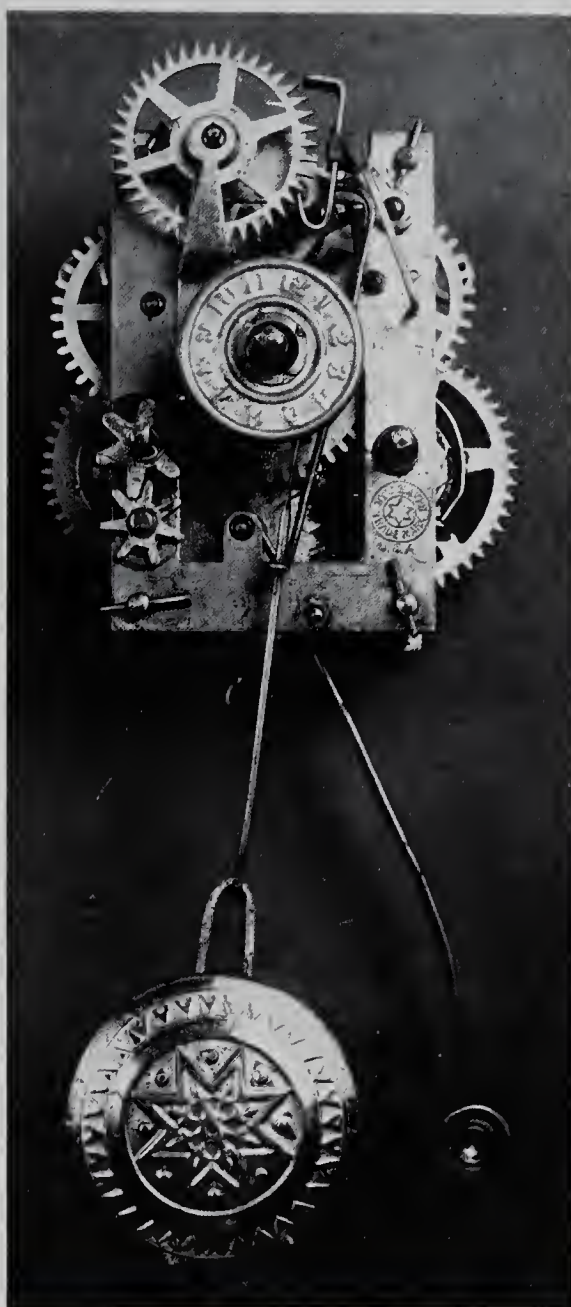
Left American Horological Industry. Movement of 'One Day Rose Cottage Time Piece' by Jerome & Co., New Haven, Connecticut. Escape wheel at front of movement; pallets formed from bent steel strip. Disc at centre for setting alarm. Frame height 3in.
