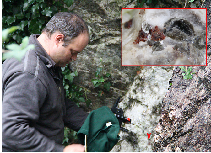
Figure 2.5. One of the authors (P.V.) performing Raman analysis on the garnets present on a pegmatite outcrop in Valchiavenna (Lombardia, Italy) using a EnWave EZRAMAN-DUAL spectrometer.
