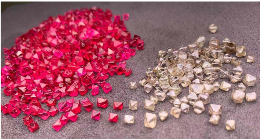
Figure 5.25. Belonging to the cubic crystal system, spinels (left) may exhibit perfect octagonal crystal habits similar to those of diamonds (right). The photo is courtesy of Xiaotao Wei.
