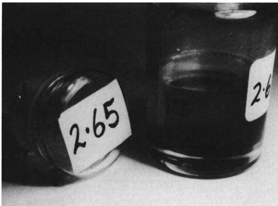
Fig. 5.4. Top: an unknown gemstone specimen being dropped into a bottle of heavy liquid having an SG of 2.65. Bottom: the unknown gemstone floats freely within the liquid, confirming that it is one of the quartz varieties
