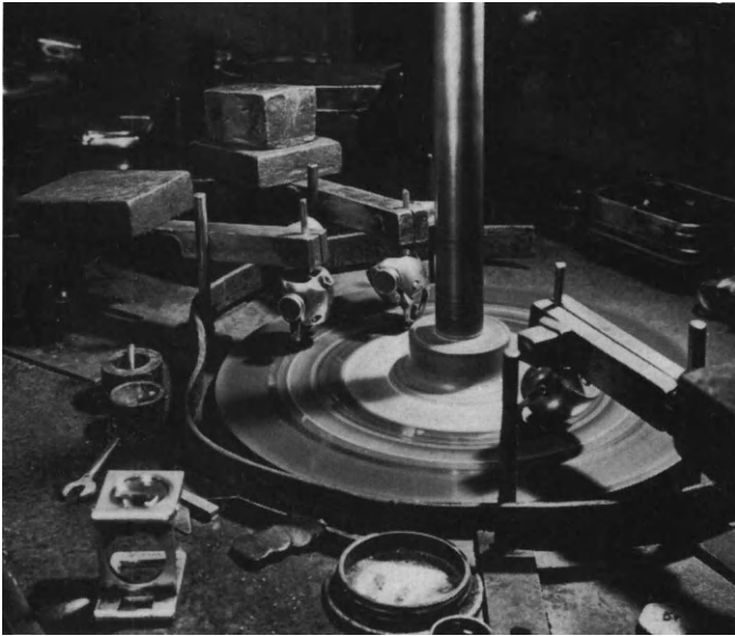
Fig. 7.13. A group of three diamonds being polished in mechanical dops. The dops are mounted in tongs which are weighted to produce the correct pressure between the diamond and the rotating scribe (De Beers.)
