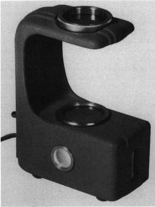
Fig. 6.10. The 'Illuminator' polariscope uses two polarising filters fixed in the extinction position. The aperture at the front can be used to provide a white light source for a refractometer (Gem Instruments Corporation)
