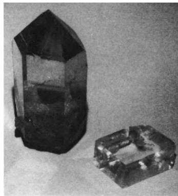
Fig. 3.6. The trigonal system. The examples of quartz (left) and calcite crystals illustrate contrasting habits in the same system. The rhombohedron shape can also be arrived at by cleaving a hexagonal shaped prism of calcite
