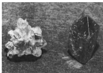
Fig. 3.7. The orthorhombic system, with examples of chrysoberyl and topaz crystals. The chrysoberyl crystal on the left is formed from triple interpenetrant twins
