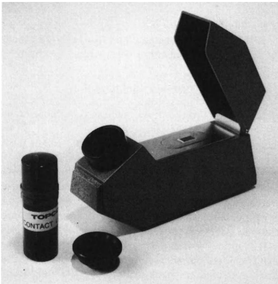
Fig. 6.5. A standard critical angle refractometer with contact fluid and polarising filter. (Gemmological Association of All Japan)
