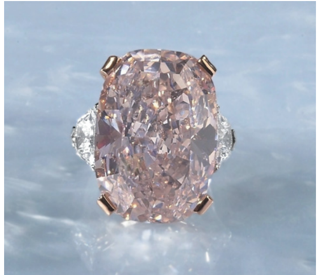
Figure 8. As indicated in figure 7, type II pink diamonds tend to be larger than type I pinks. This unusually large (50.08 ct) Fancy orangy pink diamond is a type II. Courtesy of Julius Klein Diamonds, Inc.; photo by Elizabeth Schrader.
