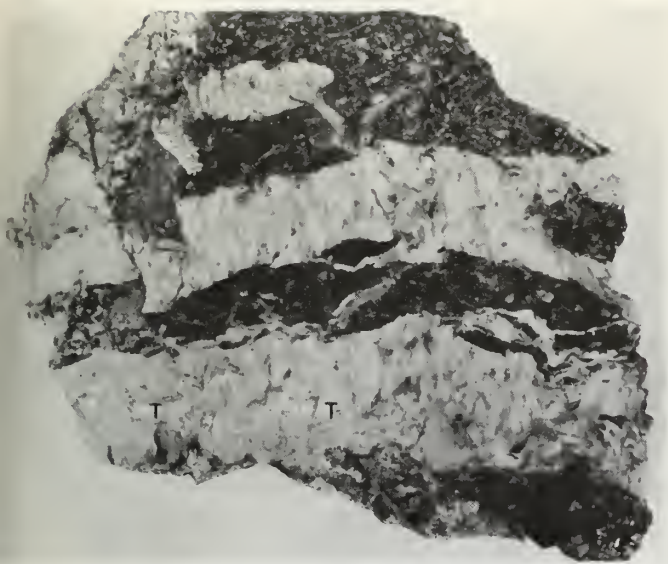
FIGURE 10A. Polished surface showing veins composed of a mixture of actinolite, talc, and chrysotile (ATC) containing fibrous tremolite (T) in sheared serpentine (S) from locality B.
