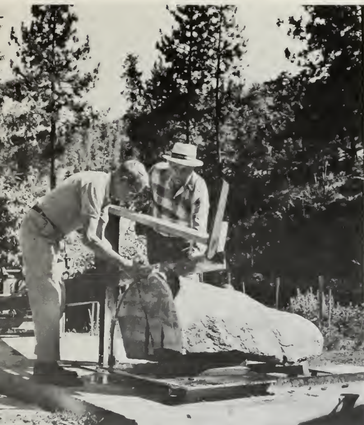
Diamond drag saw designed by George Matlack and A. C. Brill. The frame is made of I-beam steel. Power from a 3/4 hp electric motor drives the 4-foot blade. The blade has twelve 2-inch metal segments in which heavy duty commercial diamonds are soldered. The blade has an 8-inch throw, and makes a cut 40 inches long and about two-tenths of an inch wide. Clyde Call (left) and George Matlack (right) are placing the saw in operation.
