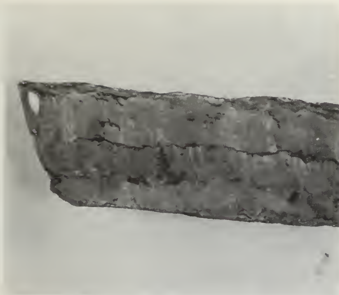
FIGURE 12. Vein of pale olive-green nephrite from locality C. The three bands of nephrite are separated by thin, discontinuous selvages of dark green serpentine. Natural size.
