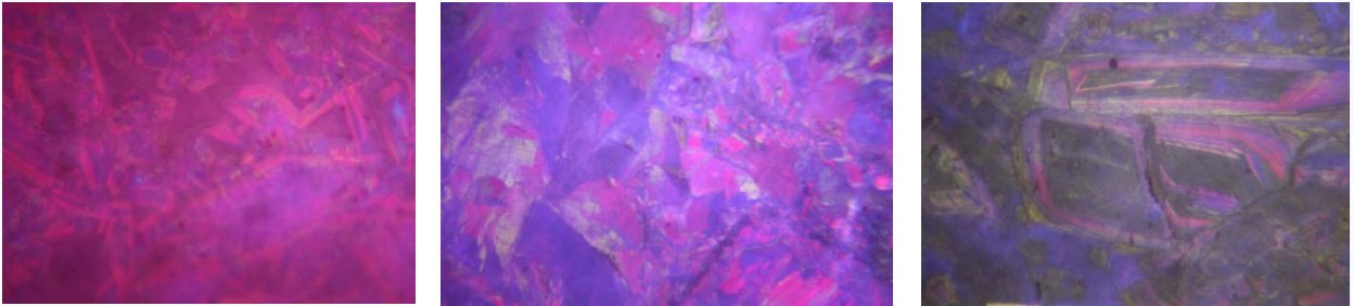
CL images of 3 different purple Fei Cui, 45X. Note that different grain sizes and zonal structures are evident.
