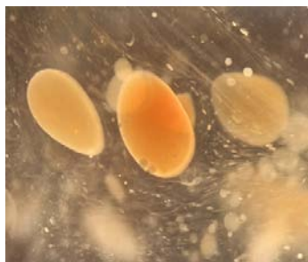
Figure 4: Patches of round-to-oval-shaped inclusions in white and yellow to brown colors ( left , Sample no. 10 magnified 6.5x; right , Sample no. 11 magnified 10.0x). Photomicrographs by Ounorn.
