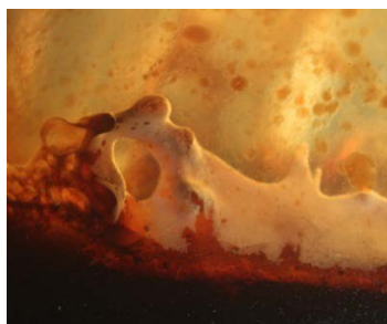
Figure 7: White material at the contact boundary between transparent and opaque parts of sample no. 2 with a zone of round-to-oval-shaped inclusions. Photomicrograph by Ounorn; magnified 6.5X
