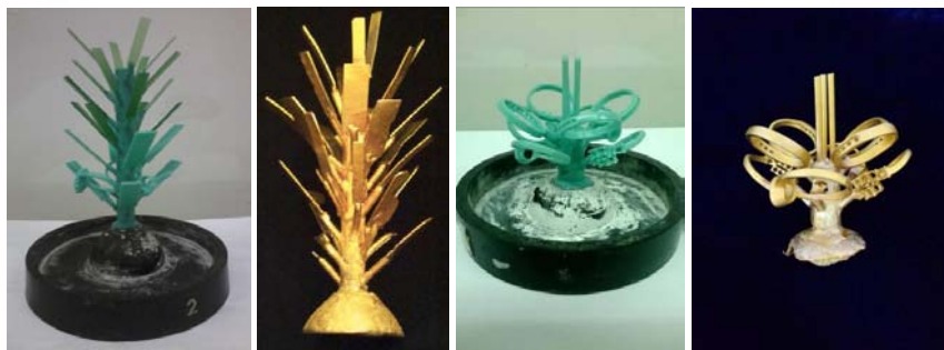
Figure 1: Typical tree set-up for lost-wax casting.
