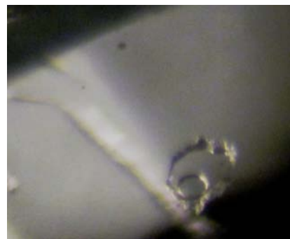
Figure 3: Cavity with 2-phase.
