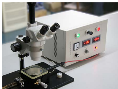
Figure1: Cathodoluminescence microscope used in this work.
