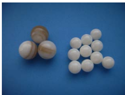
Figure 3: Bead nucleus made of freshwater “Triangle” mussel shell. Colored nucleus ( left ) is bleached by Rongalite.
