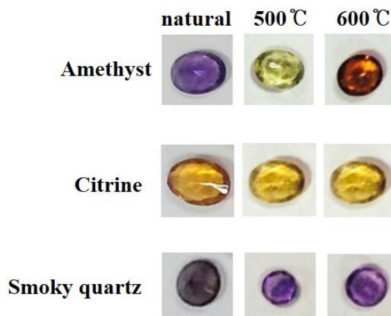
Figure 3: The quartzes samples change of color before and after heat treatment.
