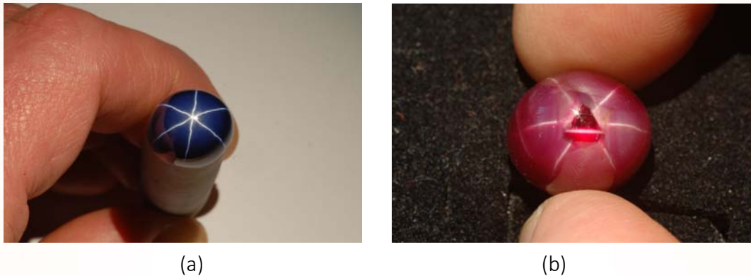
Figure 4: a (left) Synthetic star sapphire, Verneuil boule, 42 gms. and b (right) Star ruby, glassfilled, Madagascar, 9.80 ct. Photo by M.P. Steinbach.
