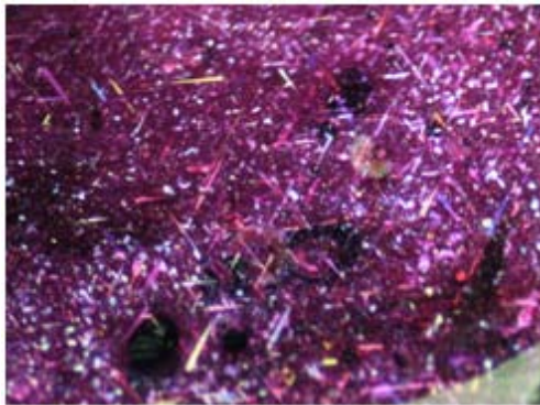
Figure 5: Brilliant colors of very finely short rutile silks in Vatomandry ruby. Photomicrograph by T. Sripoonjan; magnified 15X
