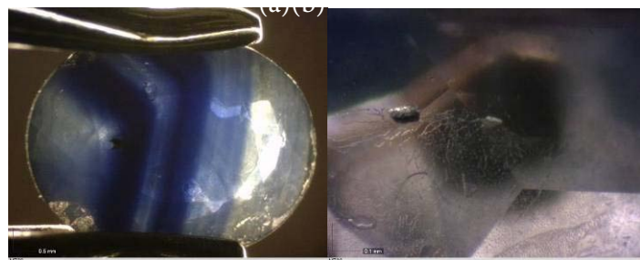
Figure 3: (a) Crystal inclusion, minute particles and colour zoning and (b) crystal and fluid inclusions in sapphire samples from Phrae.
