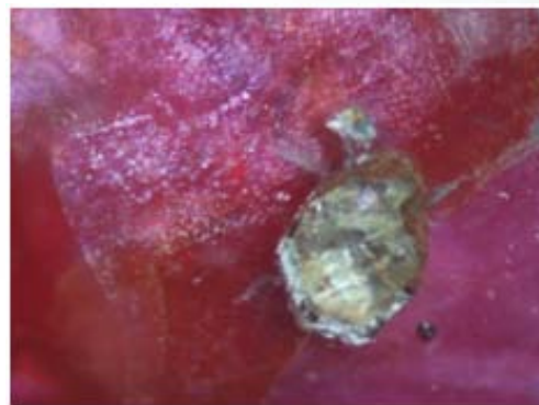
Figure 14: A quartz inclusion (confirmed by Raman Spectroscopy shown in Figure 15) rarely found in ruby from Antsirabe. Photomicrograph by N. Nilhud; magnified 40X
