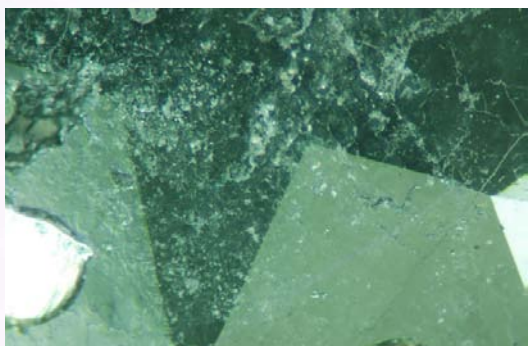
Figure 3: Fissures show black carbon like staining probably graphite (20x under reflected lighting).
