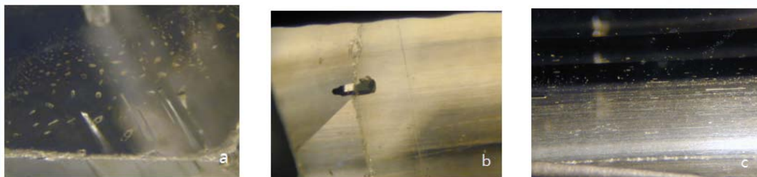
Figure 3: Photograph of the characteristic inclusions. a) healed fissures with two-phase, b) crystal pyrite, c) silk-like sodic plagioclase (albite, oligoclase).
