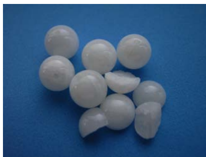
Figure 2: Bead nucleus made of Giant clam. It is cracked when drilled.
