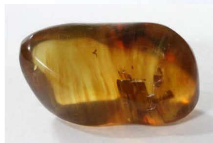
Figure 5: Swirly brown inclusions aligned in zonal pattern (Sample no. 9). Photo by Jakkawanvibul.
