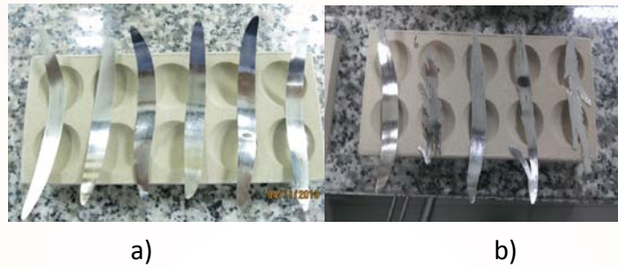
Figure 3: The gold and silver rolling sheets obtained at a) 1,050°C and 1,100°C and b) 1,000°C
