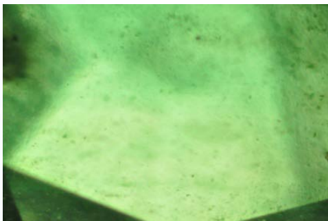
Figure 3: Most of the Jharkhand emerald appeared hazy due to presence of minute mineral inclusions. Photomicrograph by G. Choudhary, magnified 32x
