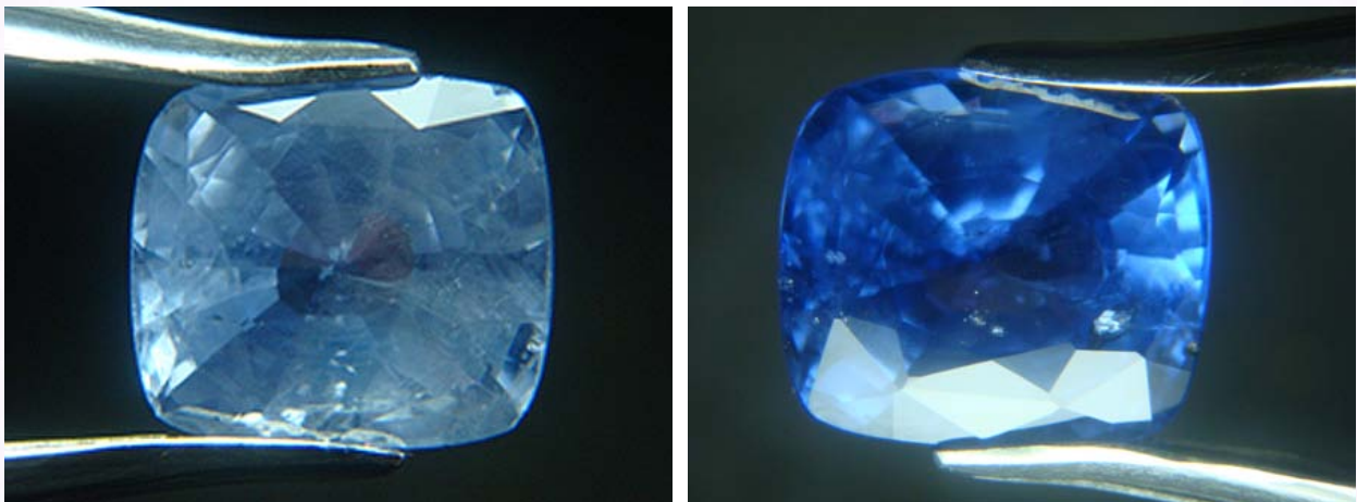
Figure 2: These two illustrations show the sample before (left, light blue color) and after (right, blue color; 6.55 ct) treated by HPHT apparatus.
