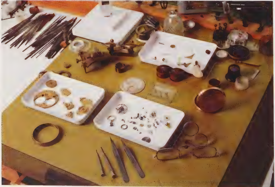
Detail of raised finishing areas showing the watch illustrated in Plate 39 at an advanced stage of production. The parts are ready for assembly and examination prior to final finishing and gilding.
