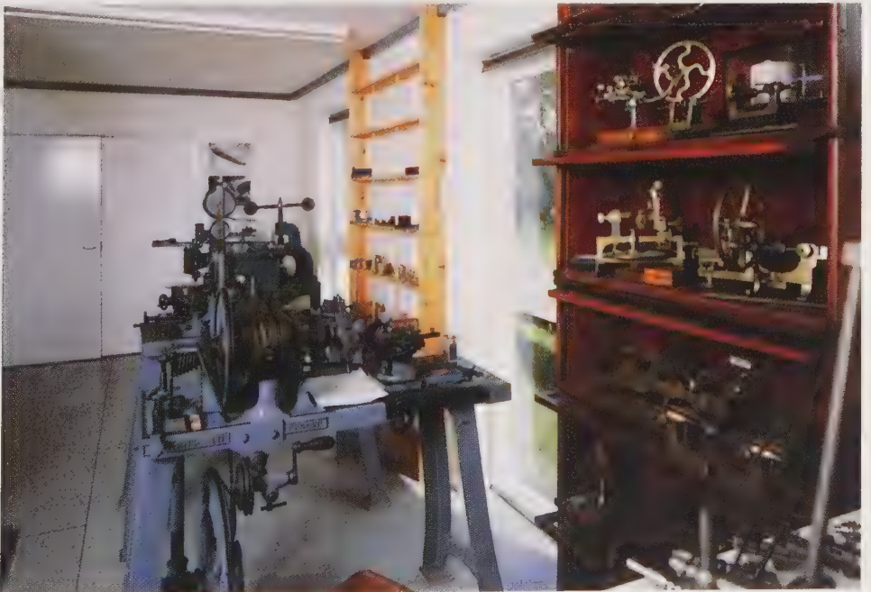
Detail of north-east corner showing engine-turning machine, pantograph milling machine, case-making press, rolls and anvil. The antique brass tools and engines can occasionally be very useful and were at one time the everyday tools of the watchmaker.
