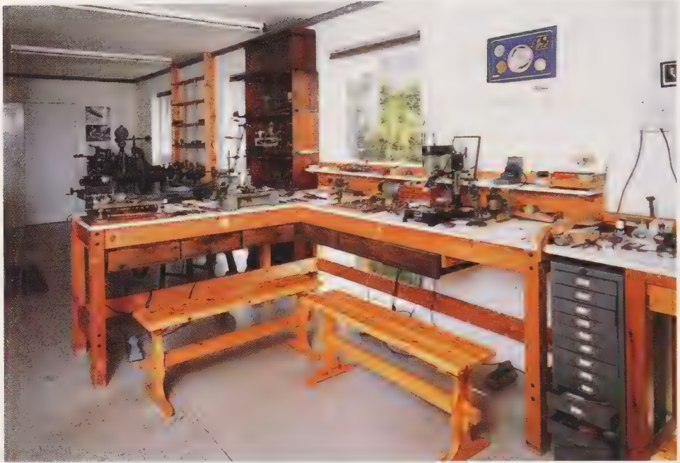
East wall looking north, showing small work benches with 8mm lathes, jewellery lathe, large and small drilling machines.
