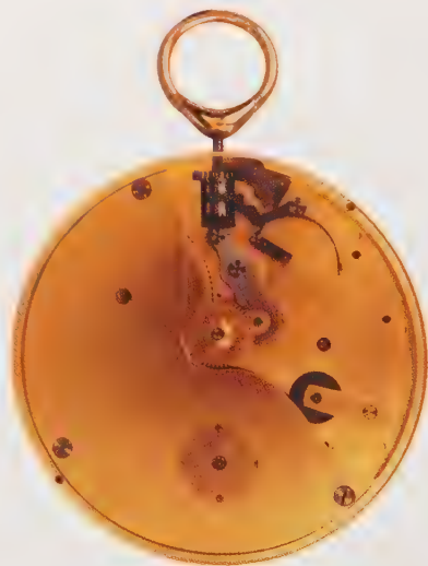
Under-dial view showing the three-position winding mechanism.
