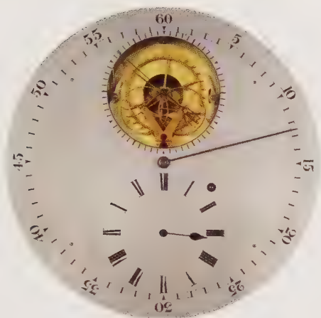
A Daniels' Grasshopper escapement fitted to a 19th-century domestic regulation
