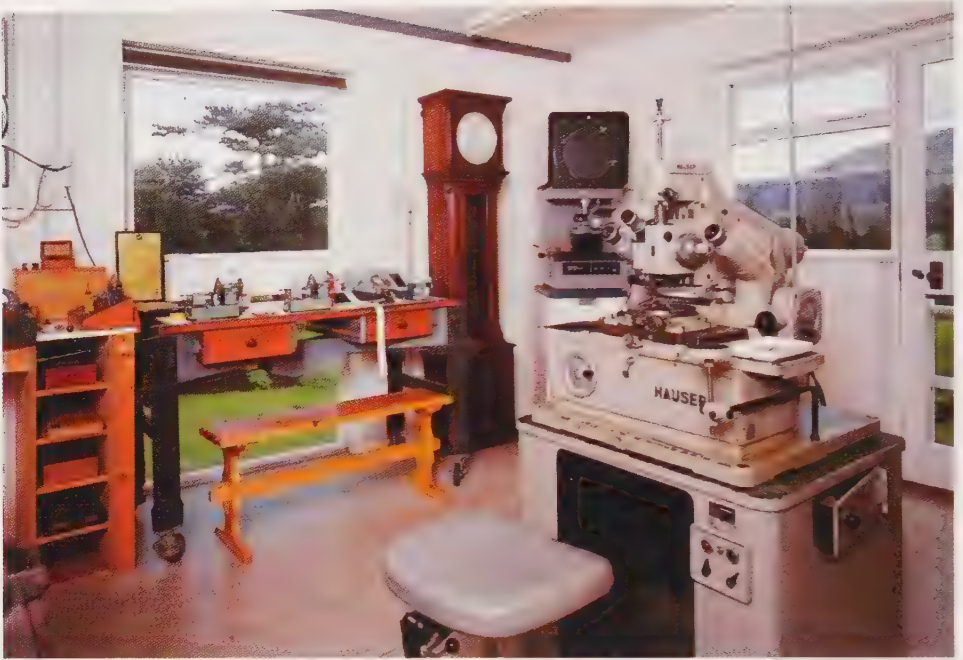
Detail of south-east corner showing optical comparator and jig borer for small, high-precision work.
