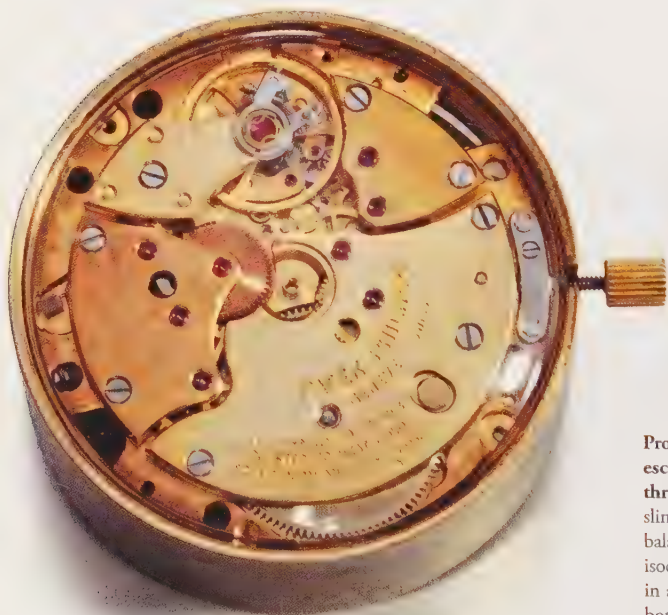
Stainless-steel automatic wristwatch with date, Rolex, Oyster Perpetual, Datejust, circa 1985. Customised by George Daniels to use a slim co-axial escapement. Nickel movement, calibre 3135, 31 jewels, monometallic balance.
