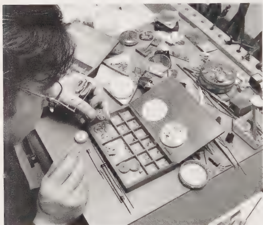
Bird's-eye views of a watchmaker's bench. Each of the components seen in the compartmented box is produced from the raw material. The case is made in 18K gold and awaits final engine turning and finishing. The completed dial lies on the lid of the box with the main plate of the movement. The tourbillon carriage, held in the left hand is complete and ready to go. At this stage the watch represents some 2,000 hours' work.
