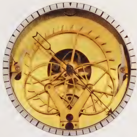
A Daniels' Grasshopper escapement fitted to a 19th-century domestic regulation
