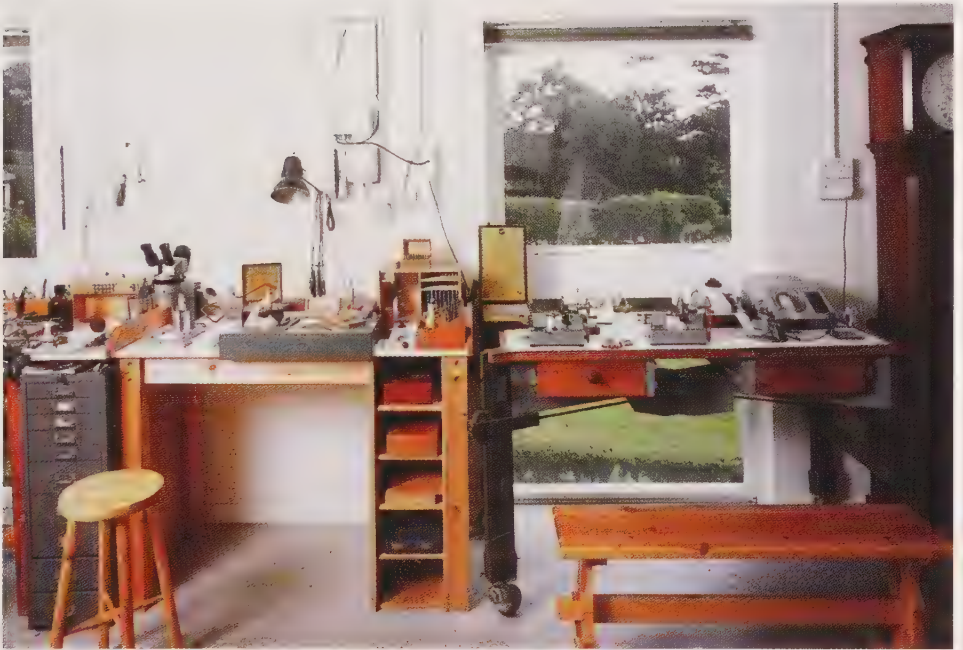
Detail of jewellery and timing benches, showing hand turns, jewellery tools, staking tools, pivot-polishing machines, timing machines for long- and short-run observations. The clock above is radio monitored to show exact GMT.
