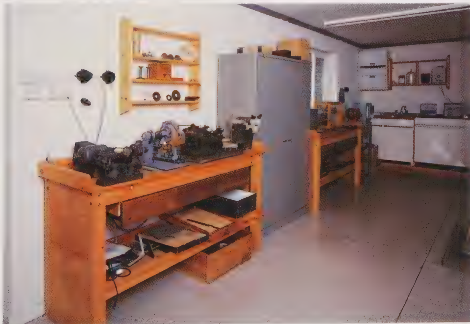
West wall looking north, showing pinion-cutting and polishing bench, furnace, wet benches with ultrasonic bath and electroplating apparatus.
