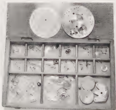
Bird's-eye views of a watchmaker's bench. Each of the components seen in the compartmented box is produced from the raw material. The case is made in 18K gold and awaits final engine turning and finishing. The completed dial lies on the lid of the box with the main plate of the movement. The tourbillon carriage, held in the left hand is complete and ready to go. At this stage the watch represents some 2,000 hours' work.
