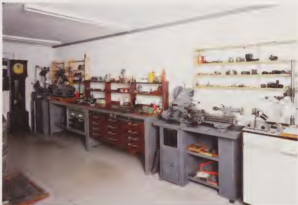
West wall looking south, showing photographic bench, screw-cutting lathe, general work benches, precision lathes for turning, wheel-cutting, etc.
