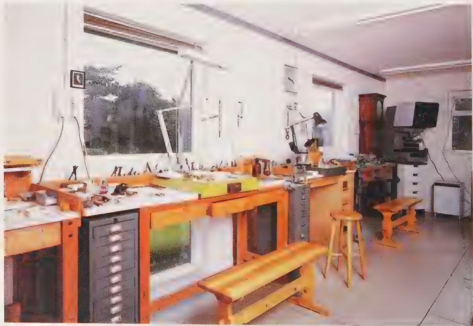
East wall looking south, showing finishing bench with raised centre, jewellery bench, timing bench, Haswell regulator, optical comparator.
