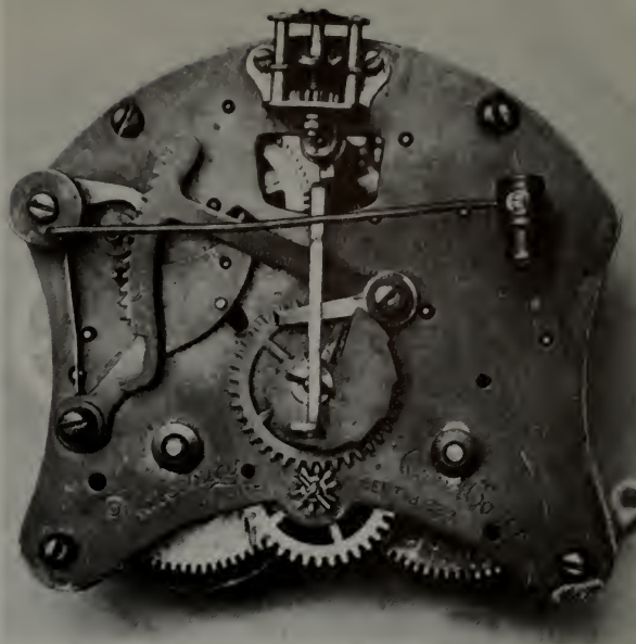
A late movement with rack strike by the Waterbury Clock Company, used in imitation-marble cases as well as other models.
