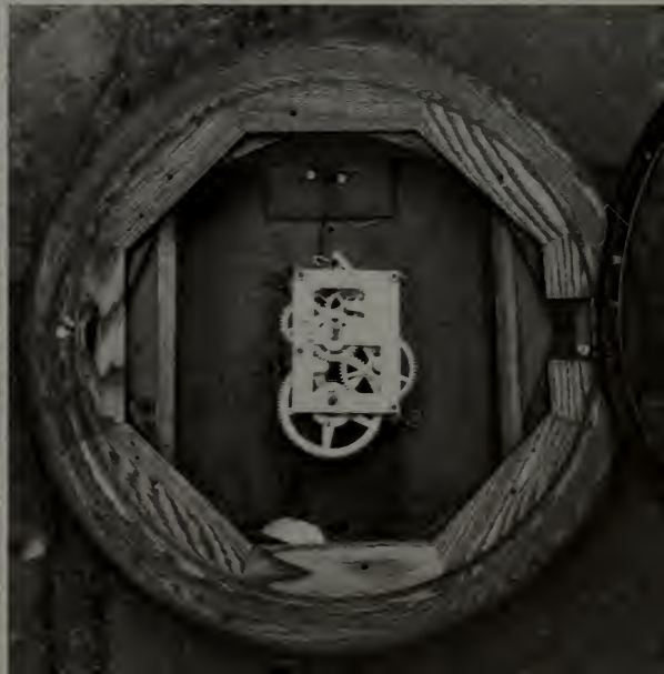
An Ansonia 12-inch dial with the escapement between the plates, the pendulum supported at the top of the case.
