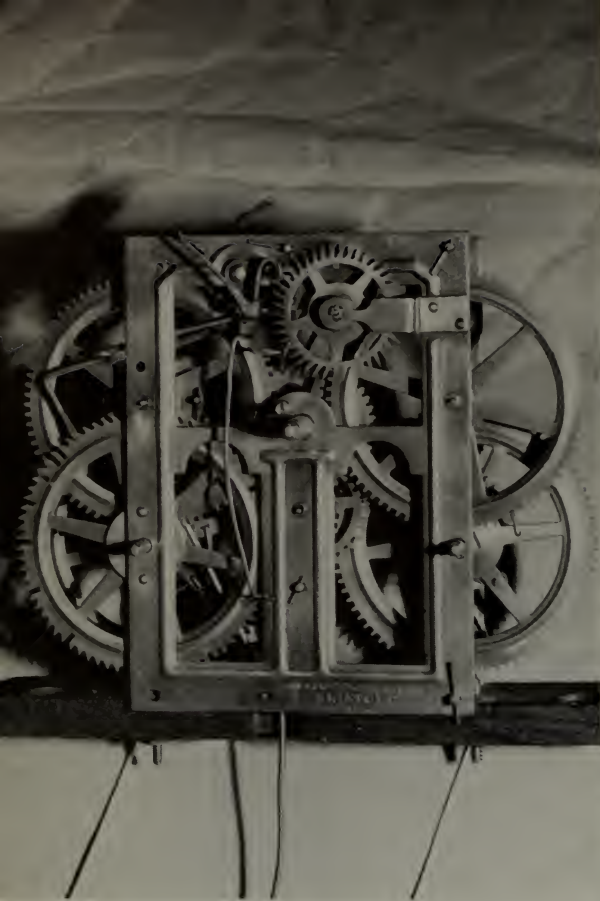
Left: The Brewster single-pin strike movement. The pin for operating the hammer is visible at the right-hand side of the cam. Right: An eight-day column clock by Birge & Fuller, 1844-8. The label contains an illustration of an early locomotive.
