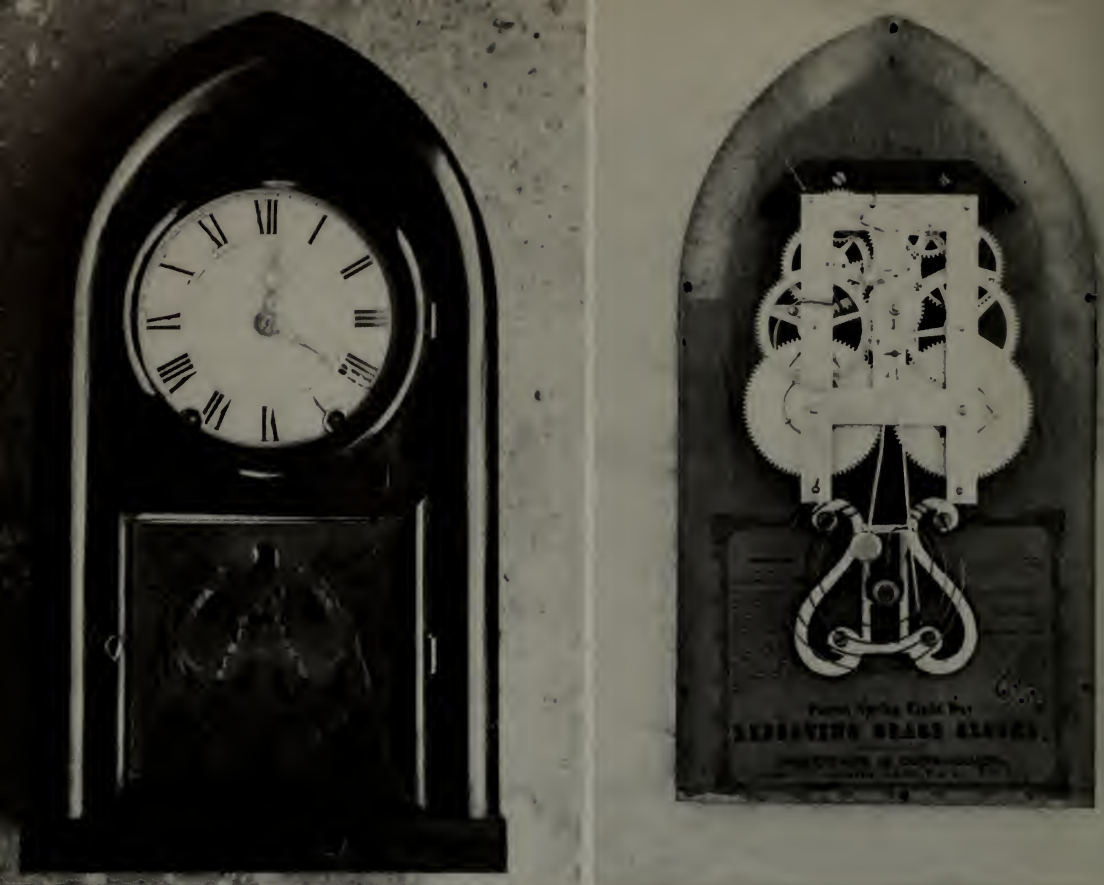
An eight-day Beehive by Brewster & Ingrahams, 1844-52. Left: Wooden dial, ground-glass tablet and brass hands. Right: The movement. Note the design of the gong-base.
