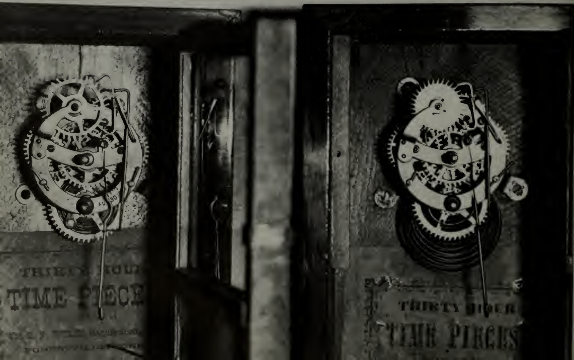
A pair of small timepieces by E. N. Welch, made in the 1870s. Above: Note that the dial of the right hand is a replacement. Below: The left of the Welch movements has B. B. Lewis's special escapement; that on the right is a normal Welch with typical solid scapewheel.
