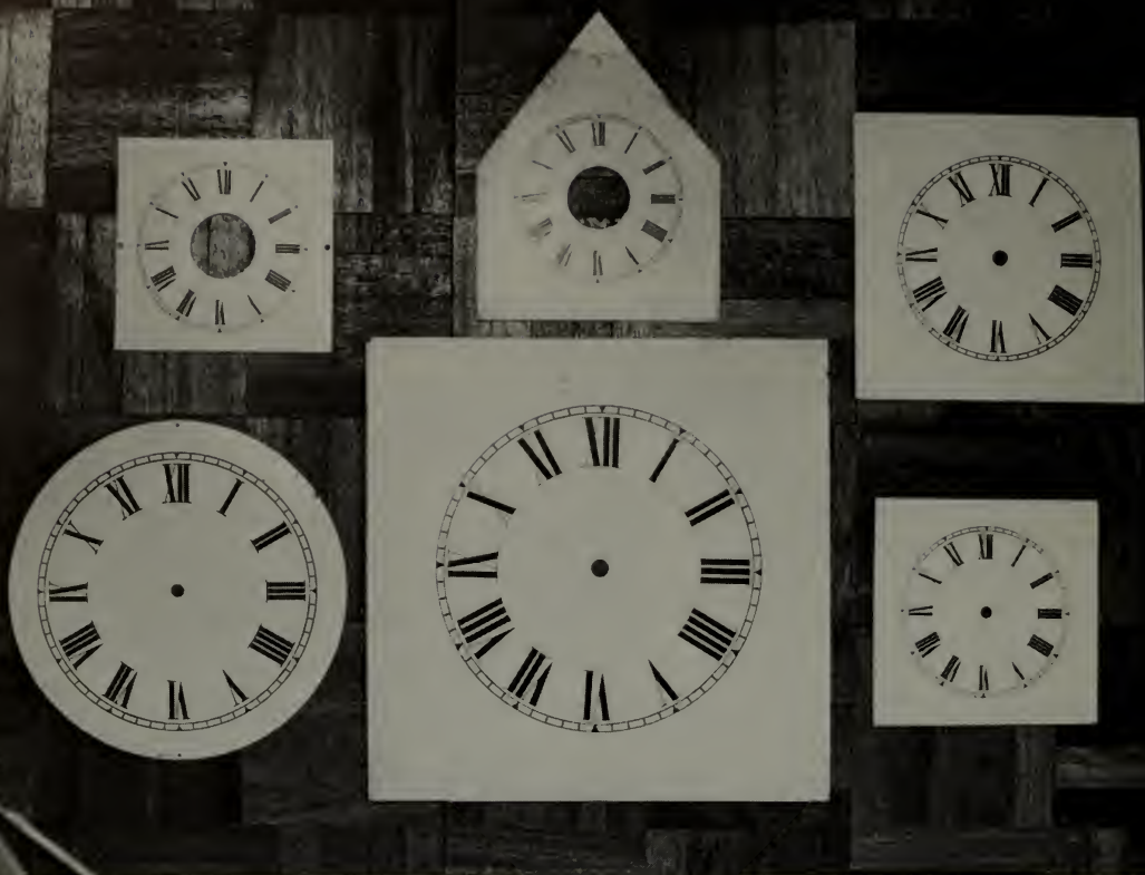
A selection of spare dials for late-nineteenth-century American clocks. No winding-holes have yet been drilled.
