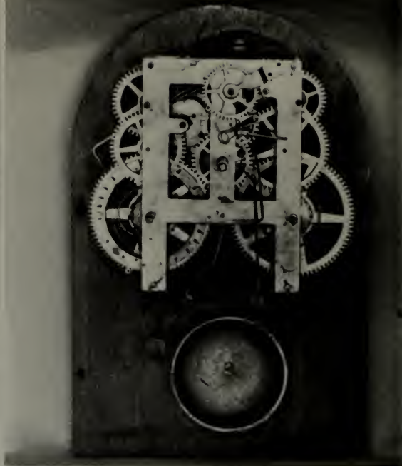
A later Holloway clock with (left) a very typical banded case. Its movement (right) is identical with that illustrated on the previous page, but it has a larger scapewheel for a shorter pendulum, and a bell-strike instead of a gong.
