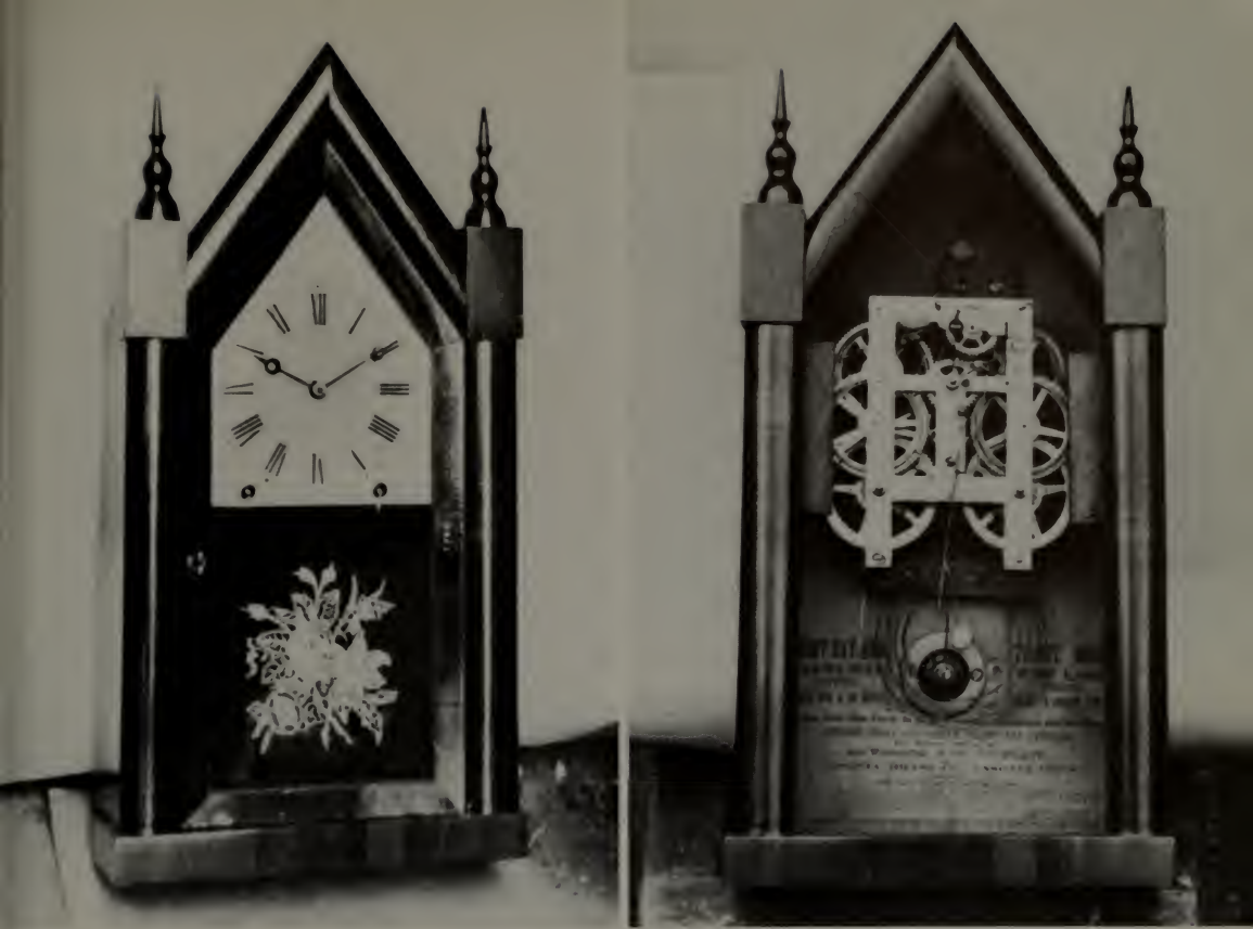
Left: An eight-day Sharp Gothic from the Ansonia Brass Company, 1854–69. Right: Its movement.
