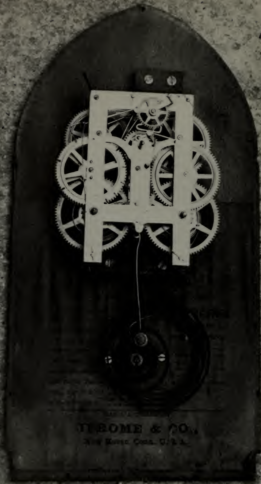
An eight-day Beehive movement by Jerome & Co (New Haven Clock Company). The 'Y' shape of the centre portion of the front plate is characteristic of this firm.
