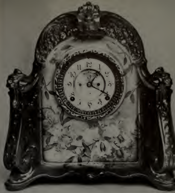
Left: A small timepiece by the William Gilbert Clock Company. The style goes back to the 1850s, but the clock is probably about 1890. The mainspring is outside the plates, facilitating its replacement. Right: An Ansonia eight-day visible-escapement movement in a Royal Bonn porcelain case, c. 1904.
