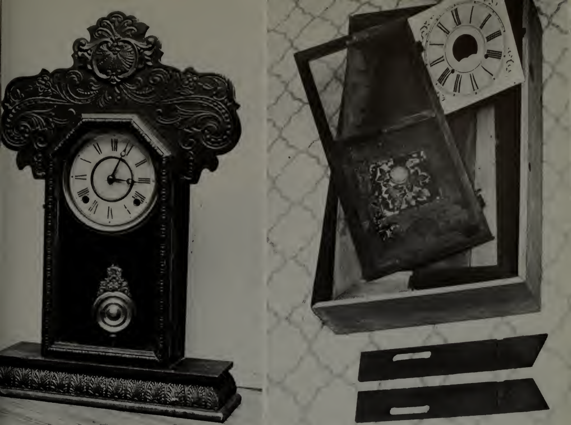
Left: An Inghram 'Oak' as found. Its side wings are missing; the mainspring has broken and spread into the bottom of the case. Right: A Brewster & Inghram's OG which was damaged by fire. The dial has been restored, and some work has been done on the case.
