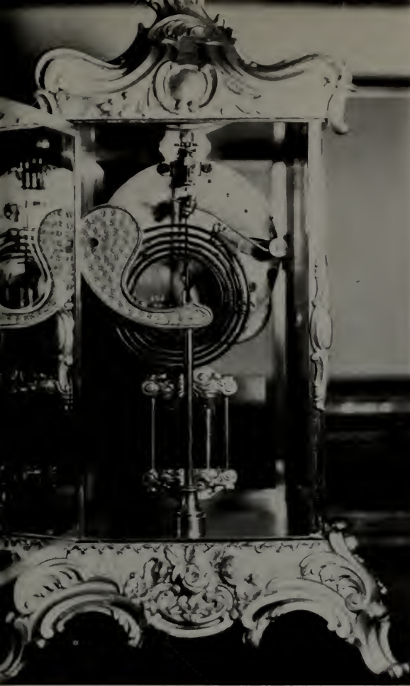
A Crystal Regulator by Ansonia, c. 1900. The rear view shows the French-type movement, rack strike and mercury pendulum.
