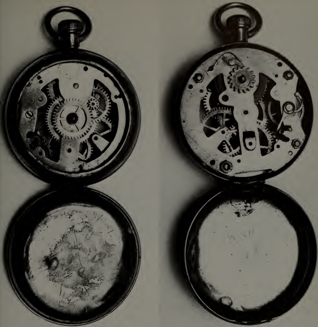
A small Waterbury clock cased to be used as a watch. Left: With the dial removed. Right: The rear side.
