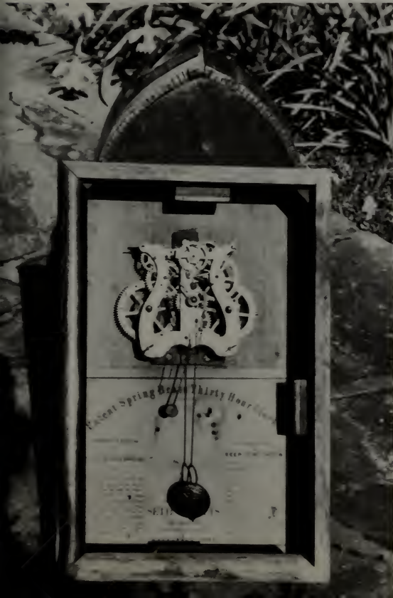
An Ansonia 12-inch dial with the escapement between the plates, the pendulum supported at the top of the case.
