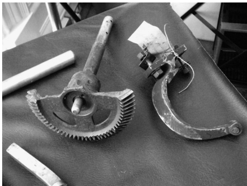
FIG 15.10 The quarter train bevel gear. The fly arbor fitted onto the spigot on this wheel. Note the damaged teeth; this was caused by the rotating mating bevel gear.
