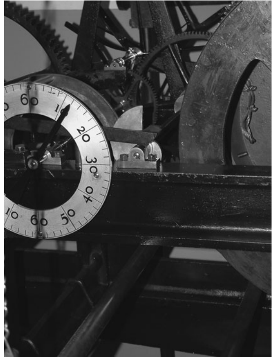
FIG 17.22 The 15-minute cam shown just after it has dropped the final locking lever.
