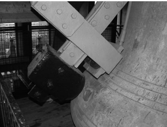
FIG 17.23 'On the lift' and well clear of the bell, the hammer is poised to make its first blow. Note the two round rubber pads that keep the hammer head just clear of the bell once it has struck.
