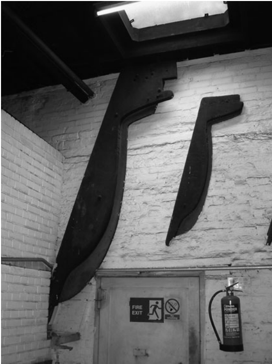
FIG 8.16 The left-hand strickle on the wall is the original pattern to make Big Ben. Acknowledgements to Whitechapel Bell Foundry.
