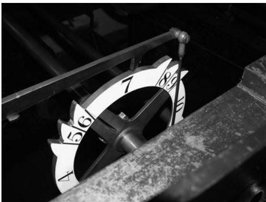
FIG 17.36 Cams fitted on the arbor signal the electric winding to turn off, to allow the quarters and hour to strike.
