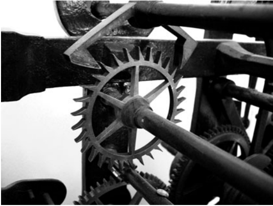
FIG 10.1 A recoil escapement.
