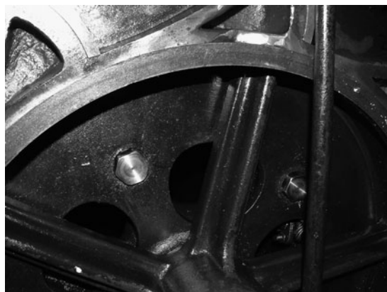
FIG 16.1 Rear view of the hour-striking barrel. The bolt heads that secure the cam wheel onto the barrel cap were found to be rubbing on the great wheel.
