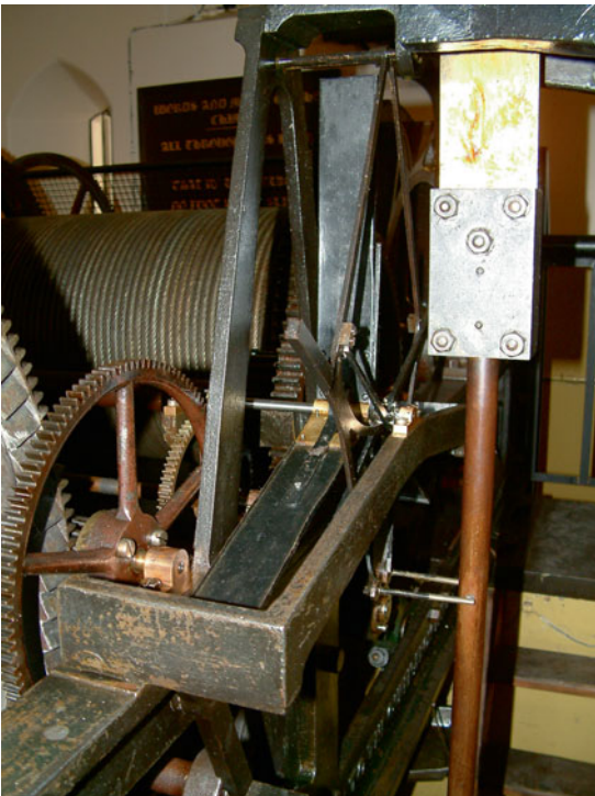
PLATE 5 FIG 2.28 Denison's double three-legged gravity escapement.
