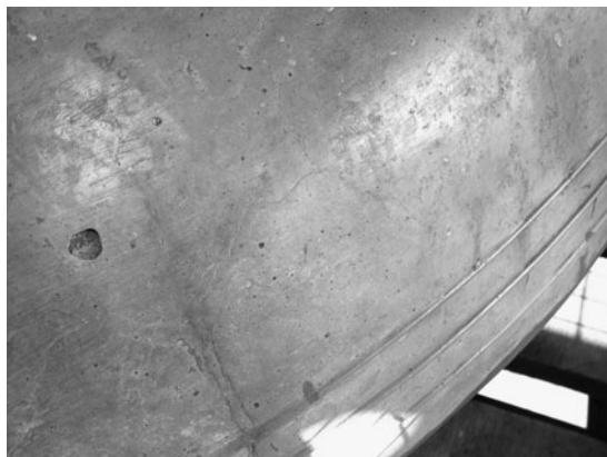
FIG 12.5 The largest blowhole in the casting and a surface mark caused by the mould surface cracking. Neither are of any significance on a casting of this size.
