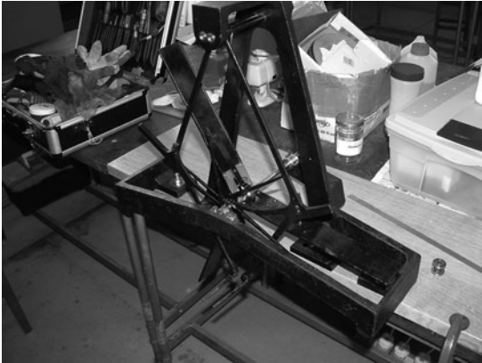
FIG 10.21 The escapement from the Great Clock, in the workshops of the British Horological Institute at Upton Hall.
