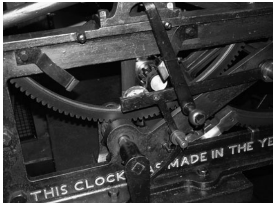
FIG 17.34 The winding-barring mechanism on the hour-striking train.
