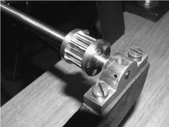
FIG 16.9 The finished lantern pinion and arbor made for the escape wheel.
