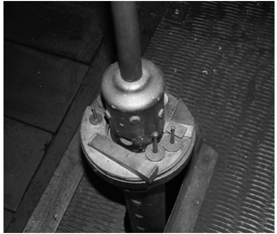
FIG 17.14 The regulation weights. The large U-shaped weight underneath is the one used for making large corrections quickly. Its counterpart, which was added to cause a gain, is now lost.
