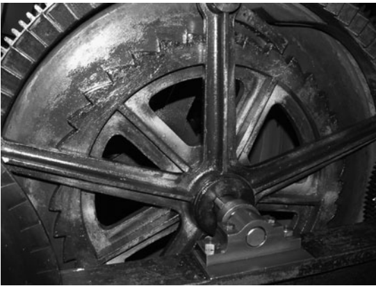
FIG 16.3 The end of the going barrel. Note the key that is one of three that retain the great wheel on its arbor. During the restoration, it was found that the boss was cracked.
