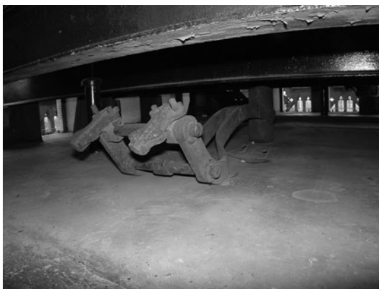
FIG 12.8 Now stored under Big Ben: the hammer that once sounded the hours on the fourth quarter bell.
