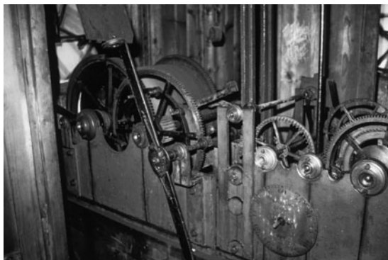
FIG 6.8 West Norwood church clock by B.L. Vulliamy, 1827. This had a 'flatbed' design, which probably originated in France.
