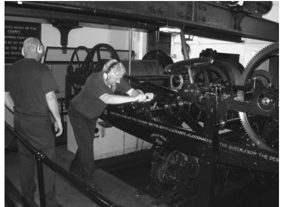
FIG 2.29 Winding the going train by hand. This figure is reproduced in colour in the colour plate section.
