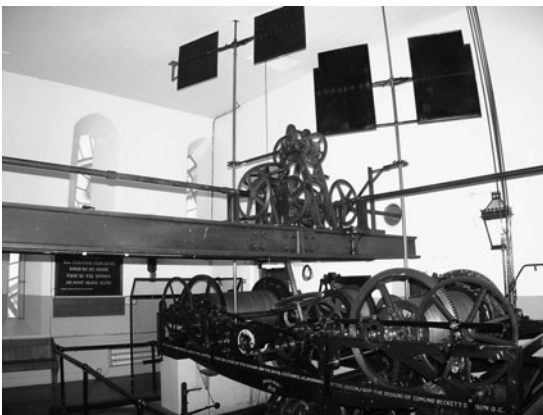
FIG 2.18 The Great Clock, showing the flies above and the connections to the dials. This figure is reproduced in colour in the colour plate section.
