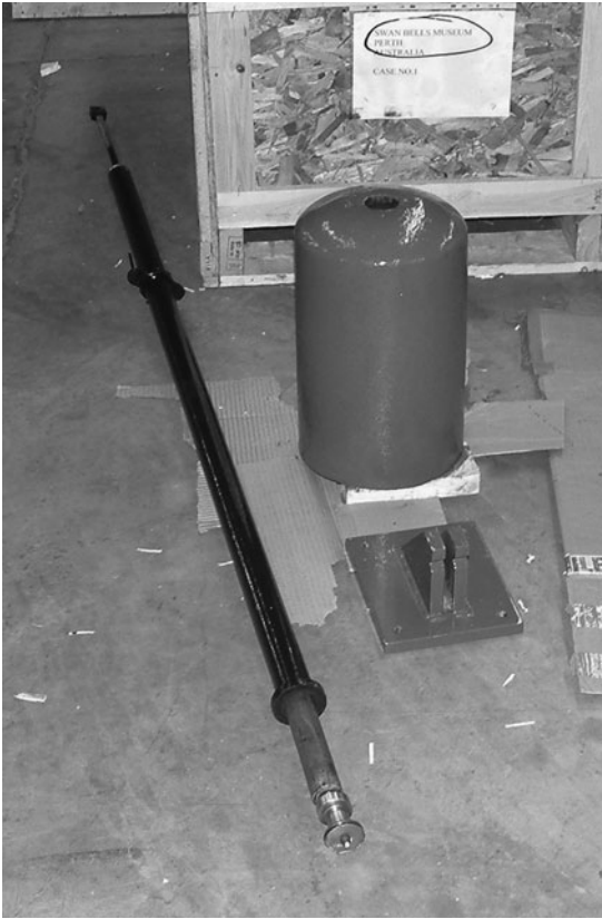
FIG 17.12 A compensation pendulum with the bob removed. The crosspiece near the top is used for regulating weights.
