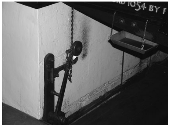
FIG 17.38 The striking train overwind switch in the set position.
