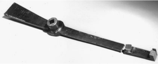
FIG 15.12 The broken locking lever. The integral leaf spring was intended to reduce the shock of locking. Courtesy of the National Physical Laboratory.
