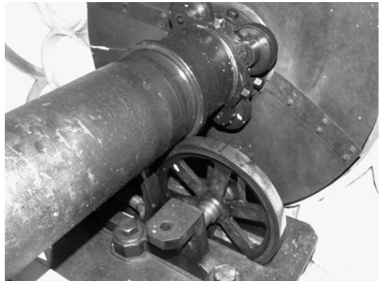
FIG 17.29 Roller bearings; the large set takes the whole weight of the hands; the small set supports the minute hand arbor.
