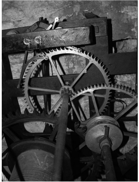
FIG 10.6 The earliest known gravity escapement on a turret clock. Harrison's detached escapement on Alkborough church clock.
