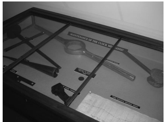
FIG 2.8 An oilcan, minute nut spanner, suspension spring, and timing record inside the display case.
