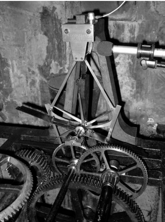
FIG 10.23 Replacement escapement by William Potts, installed in 1880.
