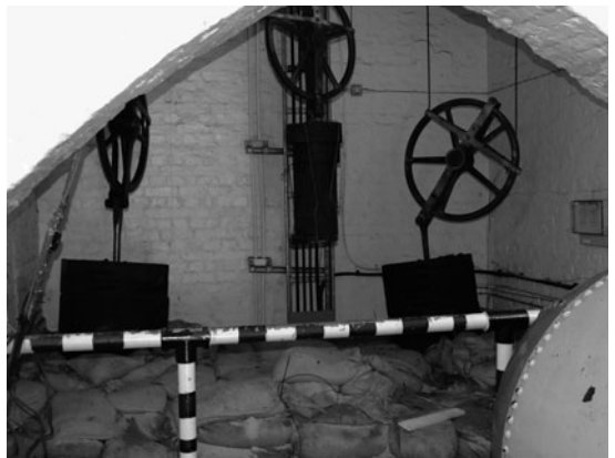
FIG 2.42 Normally the weights are out of view, but here they can be seen resting on the pile of sandbags during the 2007 restoration.
