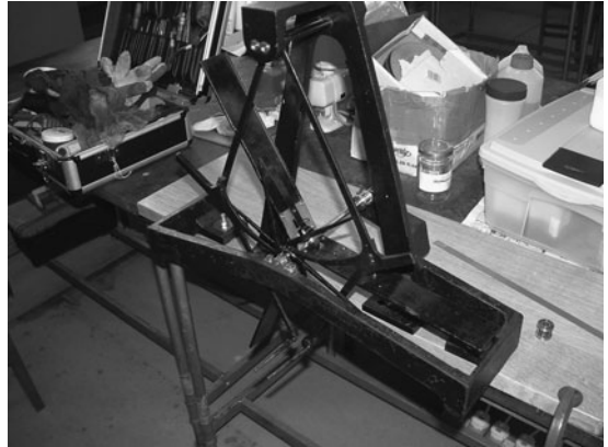
FIG 16.10 Edmund Beckett Denison's double three-legged gravity escapement. The assembly was brought to Upton Hall for the turret clock course.
