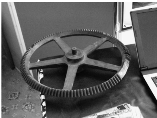
FIG 19.6 An original wooden pattern used to make castings of the bevel gears that connect the clock to the dials.
