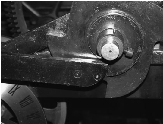
FIG 17.5 The right-hand hour arbor that releases the hour-striking train. The four-lobed cam was once part of the quarter-striking barring off mechanism.
