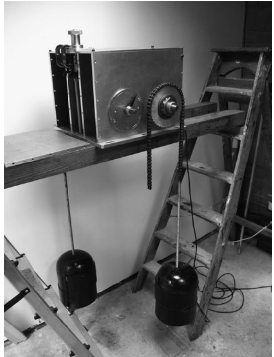
FIG 16.16 Under test, and lifting two weights totalling 2 cwt.
