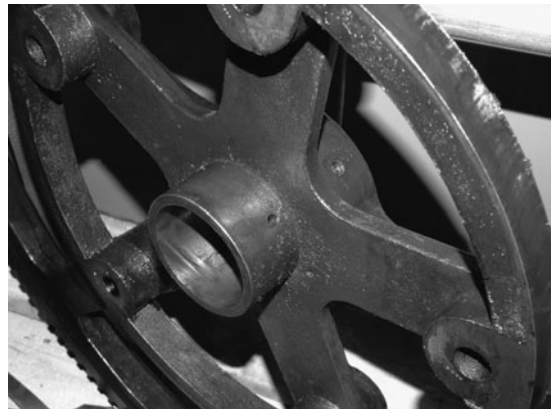
FIG 16.I3 Bush in end plate of winding wheel: note the oiling holes.
