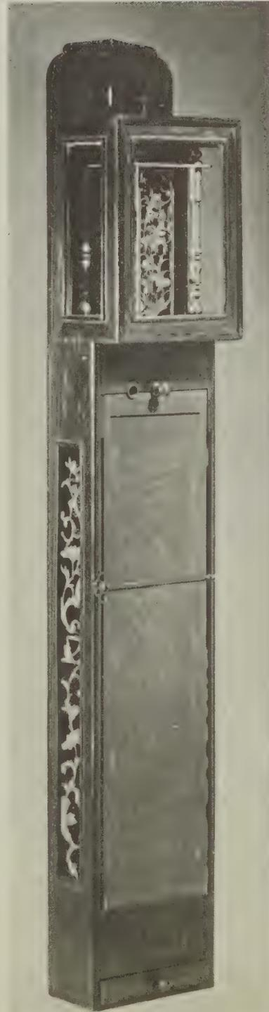
The weight moves inside a narrow pillar and a pointer, attached to the weight, projects through a slit in the front of the pillar and serves to indicate the time. The division marks are located on a groove, in which they can be slid up and down according to the variable night and day.
