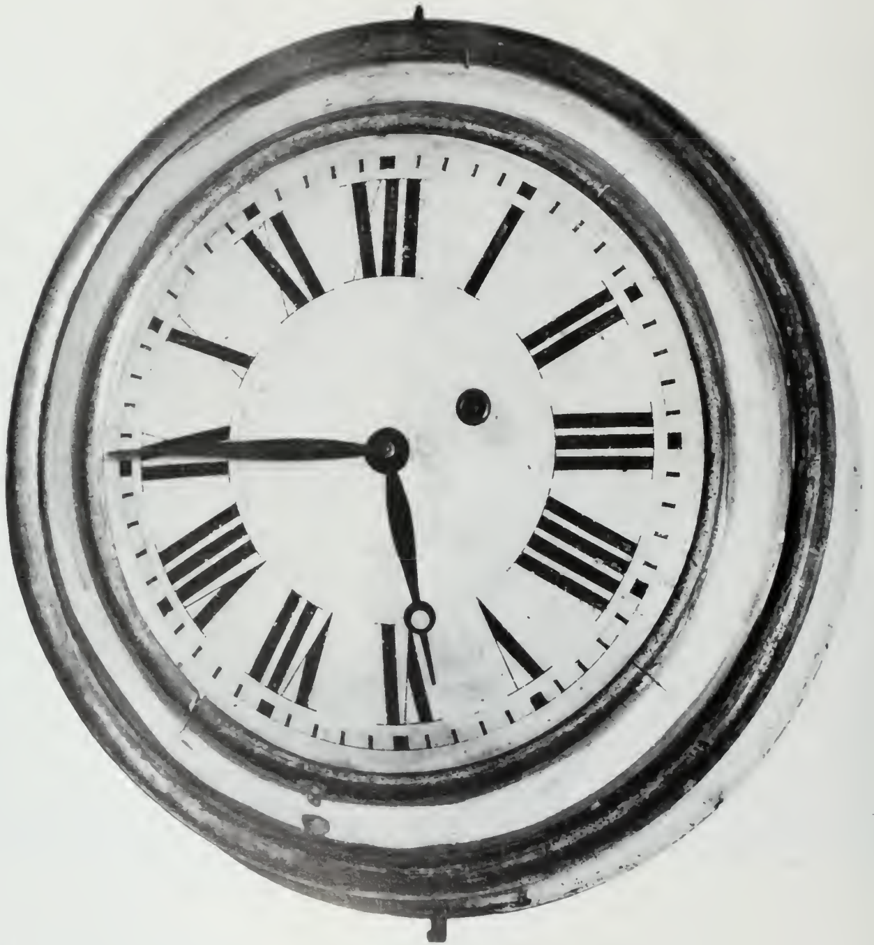
44. Brewster & Ingraham's gilt wood galleri pocket piece with an eight-day iron backplate and pendulum-controlled spring movement. The style had no dial glass. American, Bristol Connecticut, c. 1850. Private collection.
