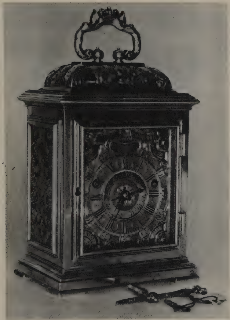
Tompion travelling clock, ca. 1700. This fine clock—which includes alarm, striking, and repeating mechanisms—formerly had arrangements whereby it could be controlled by either a pendulum or a balance wheel. Tompion made about six thousand watches and five hundred clocks during his lifetime. ( Lent to Science Museum, London, by Mrs. M. L. Gifford. )
