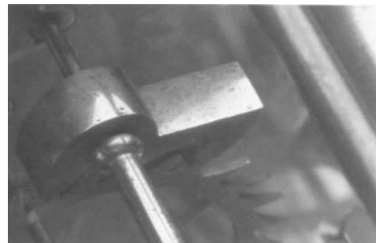
16J Detail showing the Brocot escapement.
