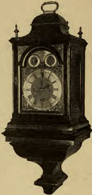
FIG. 794.—Josiah Emery, Eight-day; pull repeating quarters on six bells.
