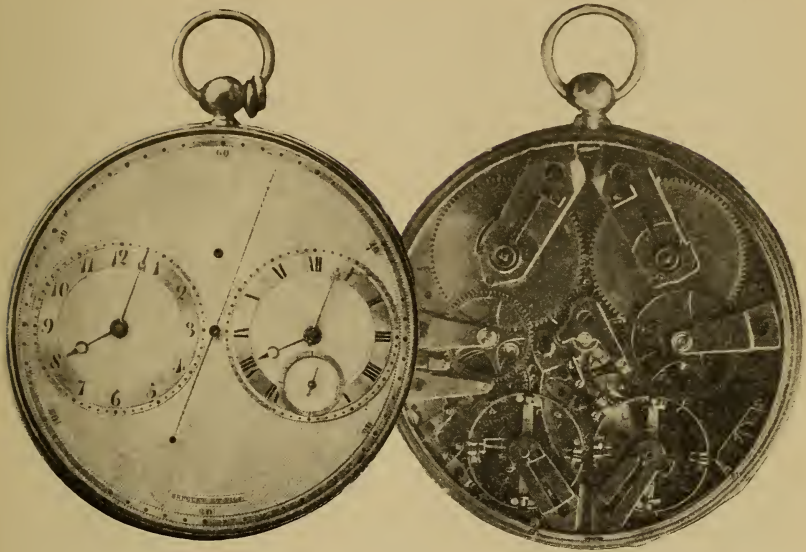
FIG. 519.—Watch with Synchronous Balances ; two Movements in one Case.
