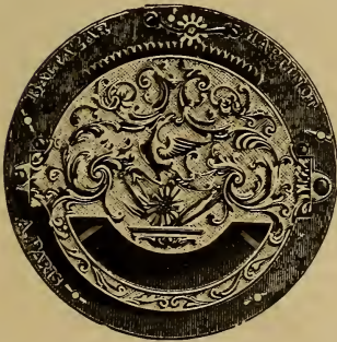
FIG. 832.—Watch, by Baltazar Martinot, showing early French arrangement of Balance-spring Regulator.
