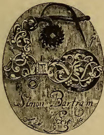
FIG. 823.—English Watch without Screws, about 1600.
