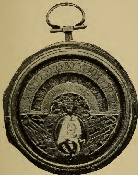
FIG. 358.—Watch with changing hour figures.
