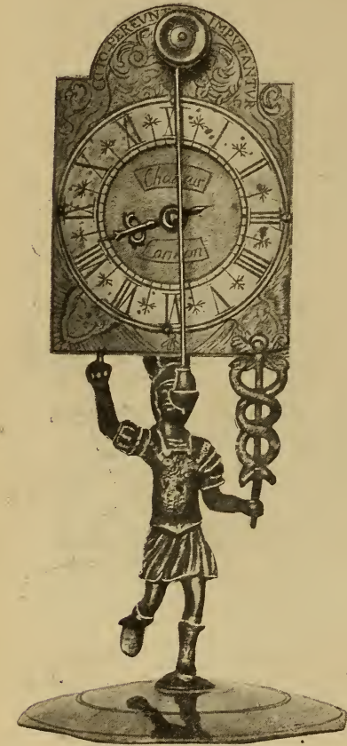
FIG. 815.—Curious little Timepiece, with pendulum in front of dial.
