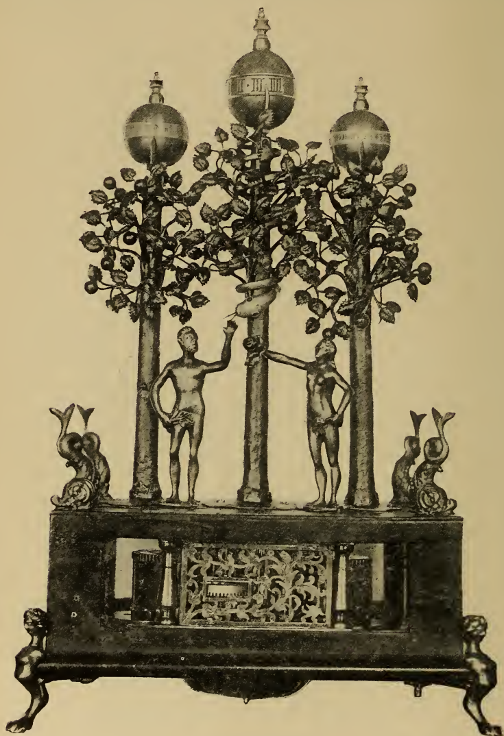
FIG. 117.—Clock with three horizontal band dials showing the hour, the day of the week, and the day of the month.
