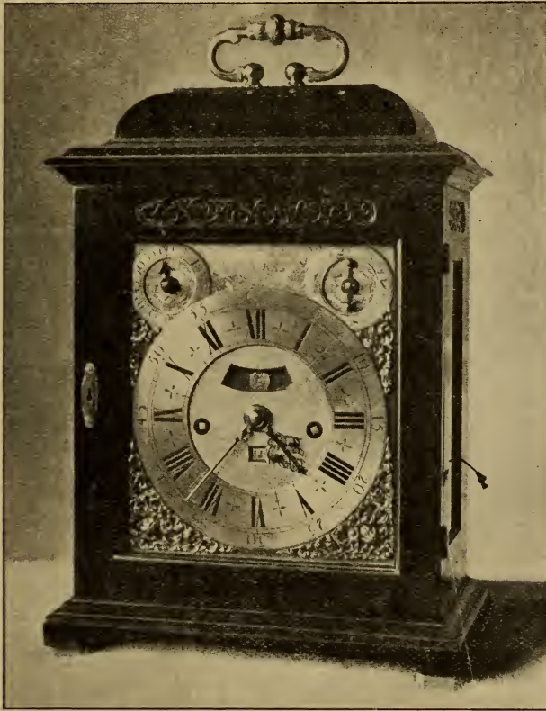
FIG. 784.—Thos. Tompion ; repeats quarters by pulling the knob and string on the right ; about 1705.
