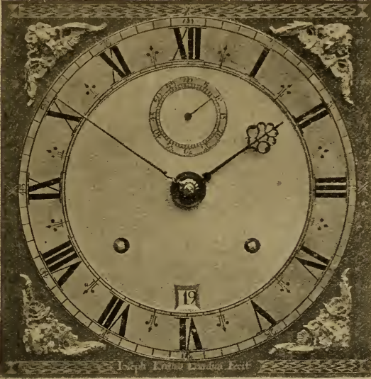
FIG. 661.—Joseph Knibb about 1685; 10 in. dial; month clock, striking on two bells.
