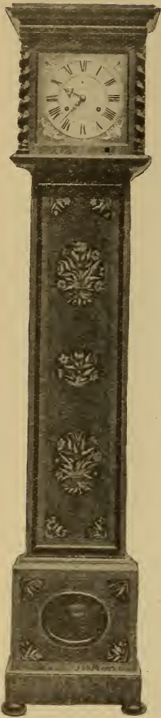
FIG. 752. — Daniel Parker, London; Month Clock, 1\frac{1}{4} seconds pendulum; door in base and glass therein; height 6 ft. 8 in., skeleton dial 10\frac{1}{2} in. square; about 1690.
