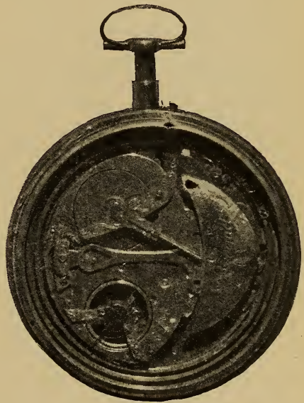
FIG. 840.—Self-winding or "Pedometer" Watch, by Breguet.
