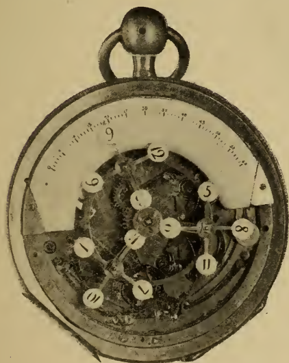
FIG. 359.—Watch with changing hour figures.
