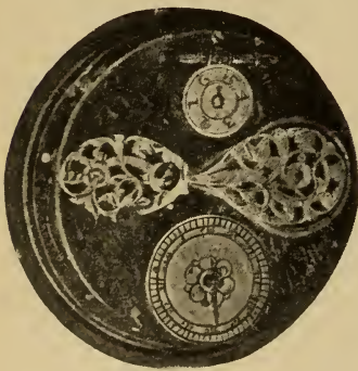
FIG. 349.—Watch with no balance spring.
