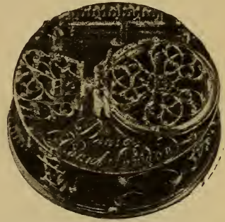
FIG. 831.—Movement with Regulator on Barrow's principle.
