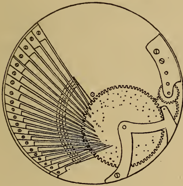
FIG. 841.— Mechanism of Musical Watch.
