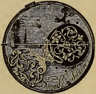
FIG. 827.—Hog's Bristle as a Balance Controller.
