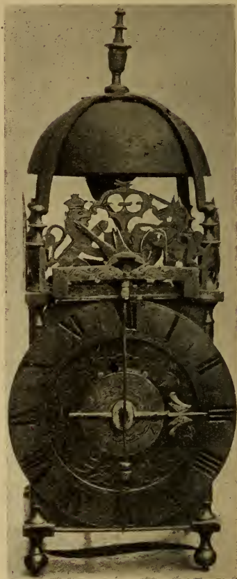
FIG. 636.—Clock with Pendulum in Front of Dial. At the head of the pendulum is the figure of a Snipe which rocks to and fro.
