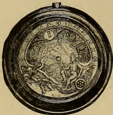
FIG. 356.—Watch with changing hour figures.
