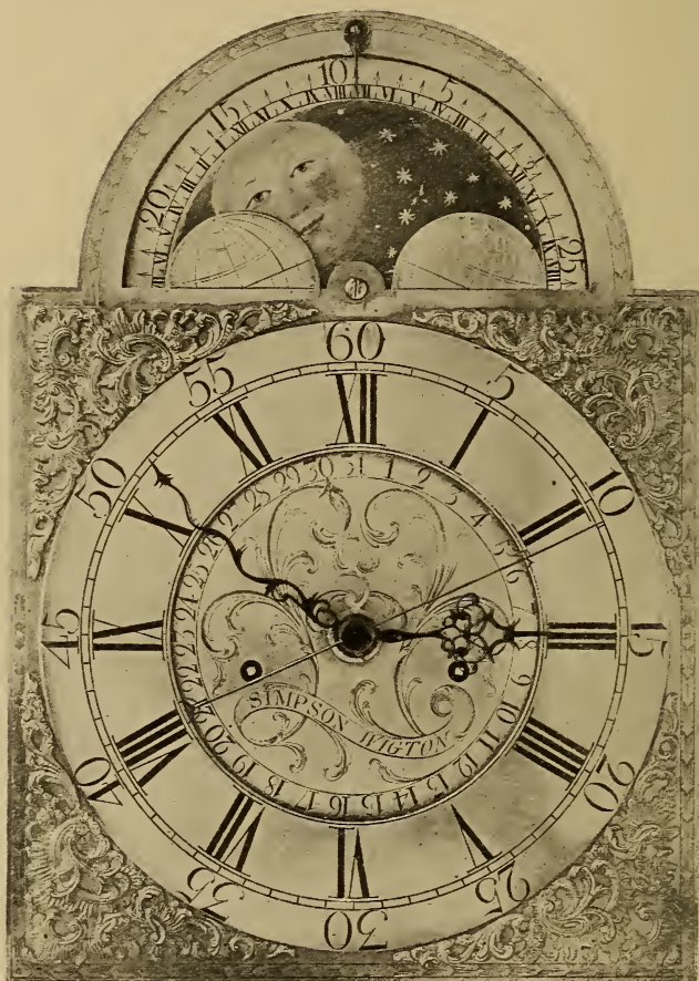
FIG. 687.—Simpson, Wigton, about 1775. Has centre seconds and day-of-the-month hands, and shows in the arch age and phases of the moon and time of high water, probably at Parton, near Whitehaven.
