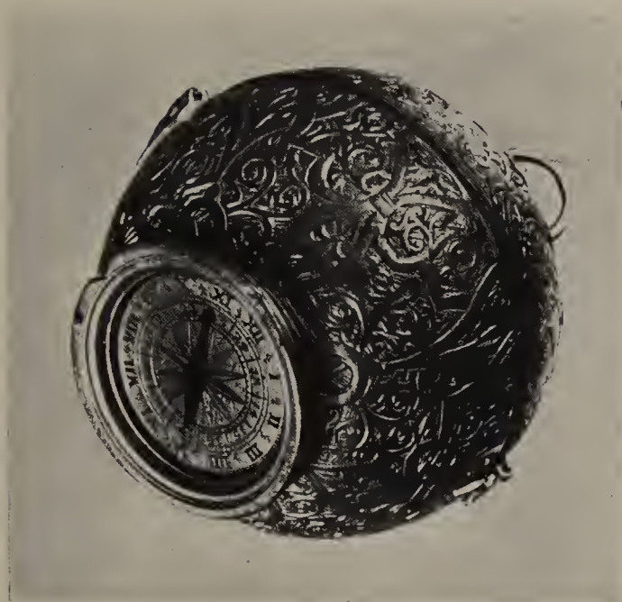
Small spherical German clock-watch, circa 1550, similar to the earliest spherical watches by Peter Henlein. The iron stackfreed movement is in two layers (striking and going trains). The mainspring has no containing barrel. The dial is at the opposite end to the pendant. The case is brass-gilt. (Ashmolean Museum, Oxford)
