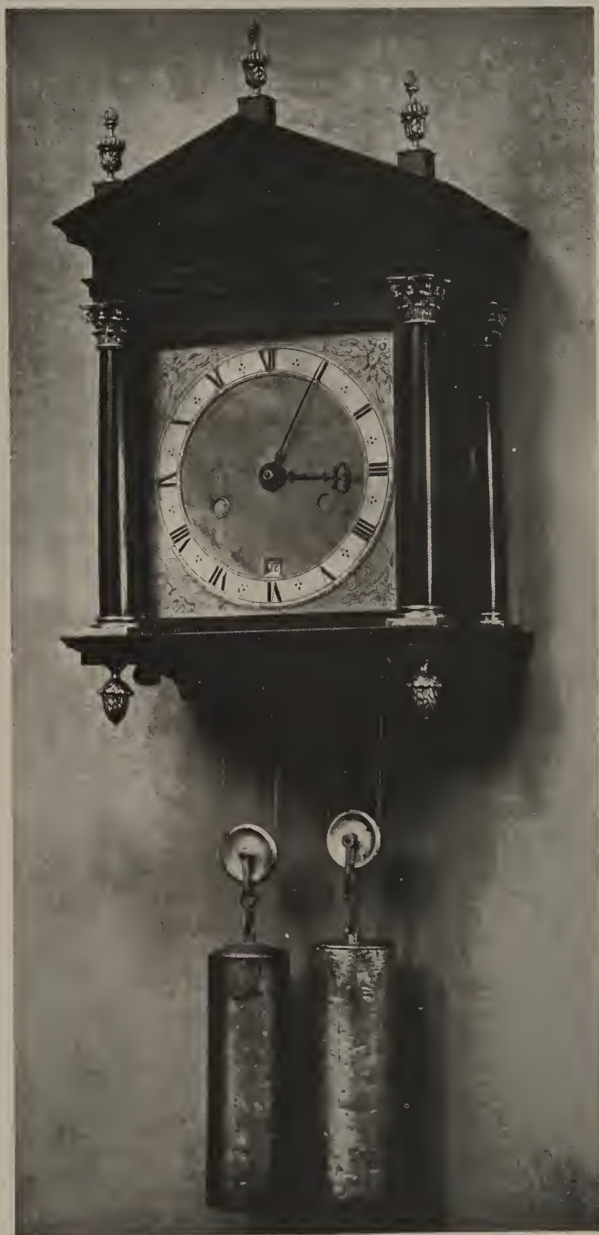
Weight-driven wall clock by Edward East, circa 1665. Note architectural treatment of case with built-up corinthian capitals; engraved dial spandrels, typical of early pendulum clocks; bolt and shutter maintaining power; brass-gilt cannister containers for driving weights.
