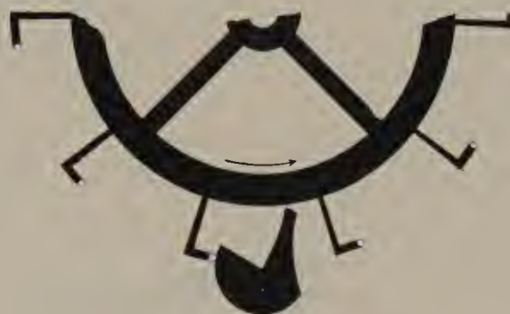
FIGURE 17. Tompion's experimental watch escapement. Pins (shown as white circles on the ends of the black teeth of the escape wheel) alternately rest on the rounded back of the balance staff roller, and impart impulse to its flat (or slightly curved) face. Impulse is in one direction only.
