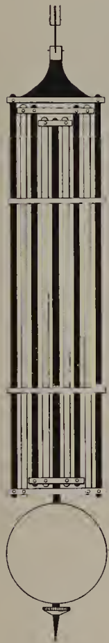
FIGURE 14. Harrison's 'Gridiron' pendulum. The five steel rods are black and the four brass rods are white.
