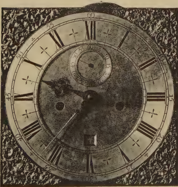
FIG. 737.—Thos. Tompion, about 1695. Month clock; 10½-in. dial bolt and shutter maintaining power.
