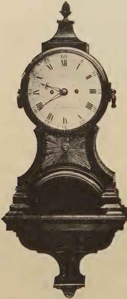
FIG. 884.—John Johnson, Ebony Brass-mounted Eight-day Balloon Clock, Pin Wheel Escapement; height, including bracket, 27 in.; about 1800.
