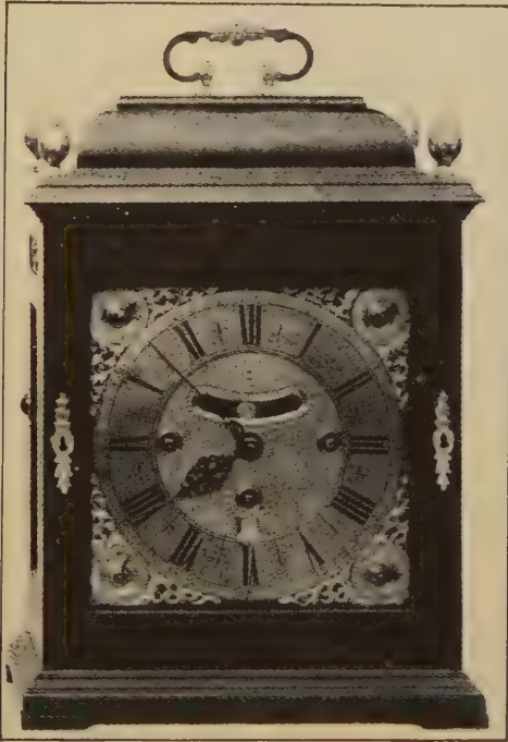
FIG. 488.—Fine Bracket Clock by Daniel Quare, chiming quarters on six bells.
