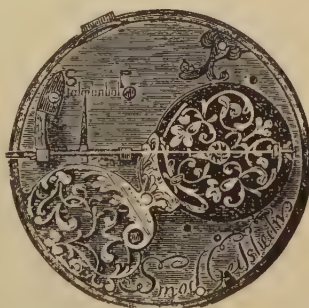
FIG. 899.—Hog's Bristle as a Balance Controller.
