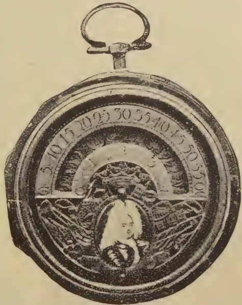
FIG. 379.—Watch with changing hour figures.
