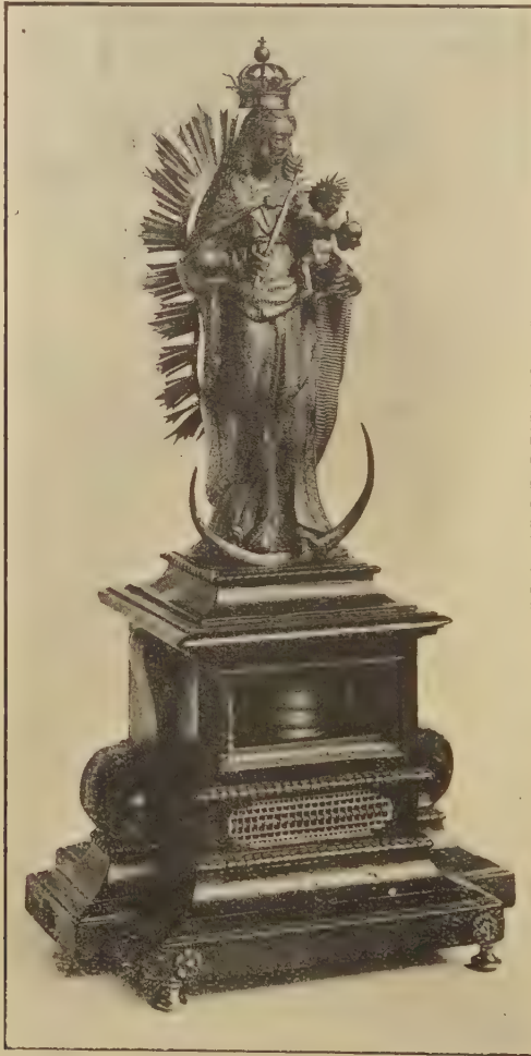
FIG. 126.—Clock with horary numerals on a revolving crown.
