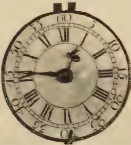
FIG. 359.—Hands of the "beetle" pattern.
