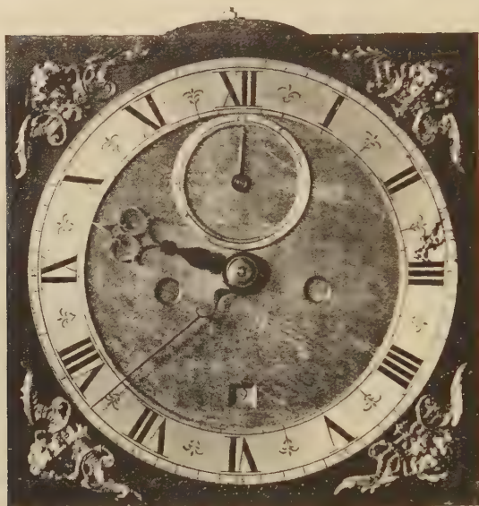
FIG. 734.—Edward East, about 1680. Eight-day clock; 10-in. dial; bolt and shutter maintaining power.
