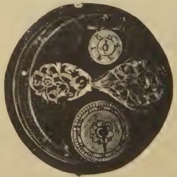
FIG. 370.—Watch with no balance spring.
