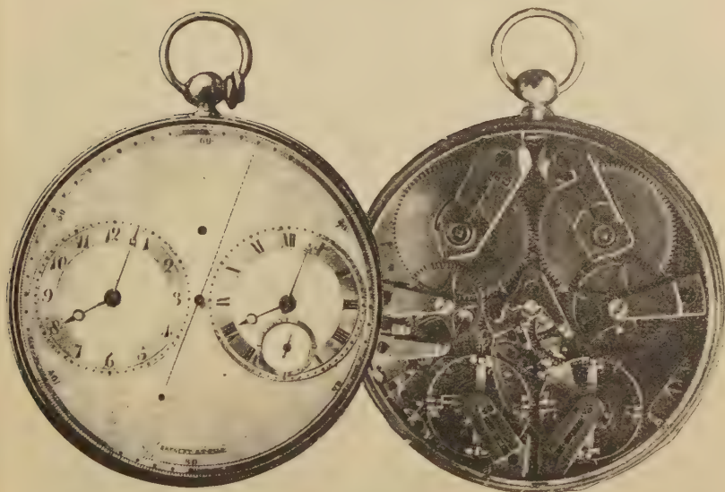
FIG. 566.—Watch with Synchronous Balances ; two Movements in one Case.
