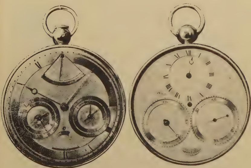
FIG. 568. Watch with Chronometer Escapement mounted in Tourbillon Carriage.
