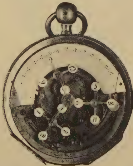
FIG. 380.—Watch with changing hour figures.
