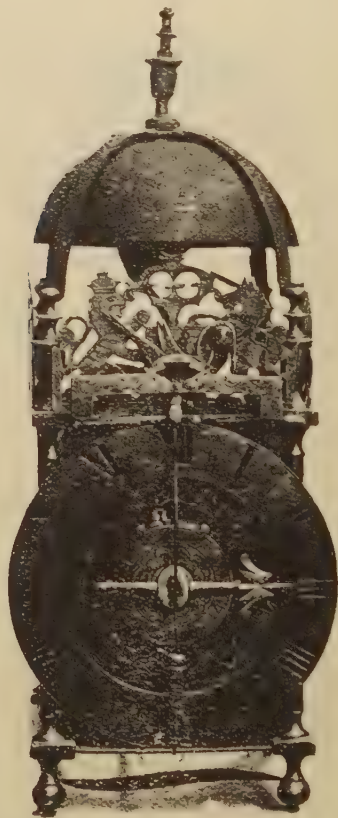
FIG. 695.—Clock with Pendulum in Front of Dial. At the head of the pendulum is the figure of a Snipe which rocks to and fro.
