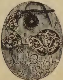
FIG. 895.—English Watch without screws, about 1600.
