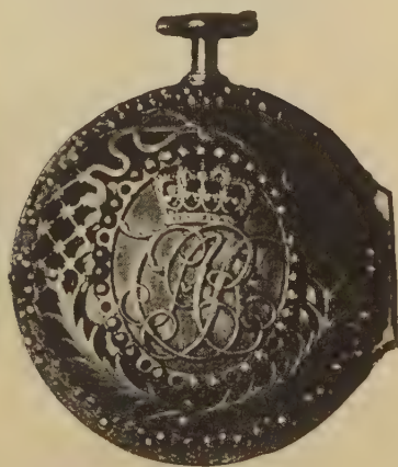
FIG. 330.—Watch by Vulliamy, with Steel Pendant and Steel Out-case pierced.
