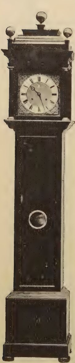
FIG. 829.—Joseph Knibb, "at Hanslop"; Month Clock, striking on two bells, as explained on p. 353; height 8 ft.; about 1705.
