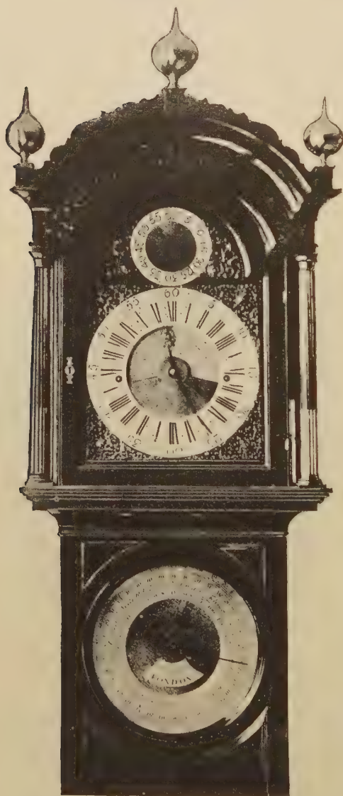
FIG. 524.—Long-Case Clock, by John Ellicott with Equation of Time Dial below the Hood.
