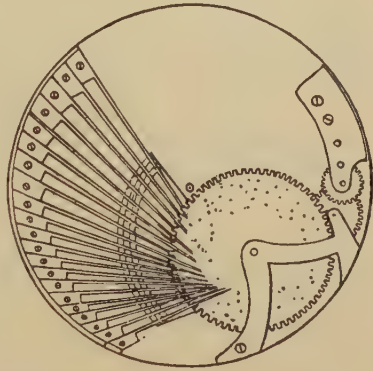
FIG. 913.— Mechanism of Musical Watch.
