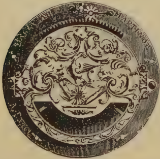
FIG. 904.—Watch, by Baltazar Martinot, showing early French arrangement of Balance-spring Regulator.
