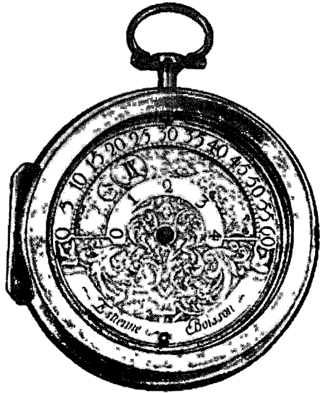
Figure 24. 'Wandering-hour' watch by Estienne Boisson, London (?), early eighteenth century. Boisson was presumably a Huguenot refugee. This type of watch gets its name from the manner of display of minutes and hours. The upper arc shows minutes, and an hour indicator (roman numerals) swings across below it, marking by its position the number of minutes elapsed since the last hour. The inner arc of numbers shows the quarters.
