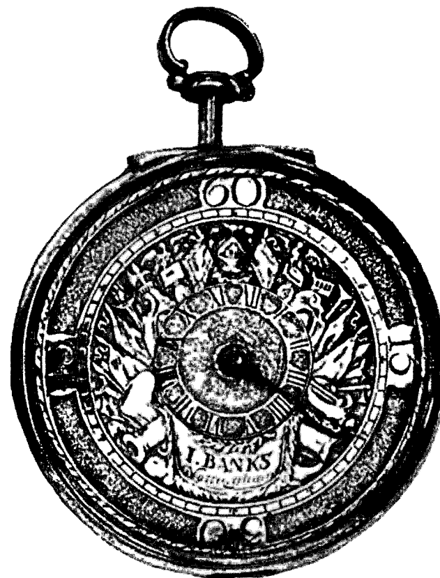
Figure 25. Watch with differential dial by James Banks, Nottingham, c. 1700. This watch thriftily shows hours and minutes by means of a single hand that sweeps two number rings. The outer ring (arabic numerals for the quarters) shows minutes; the inner (roman numerals), on a separate disc, shows hours. The inner disc turns clockwise with the hand, but slower, so that the hand gains and moves on to the next numeral every hour. The time shown is 3.20.
