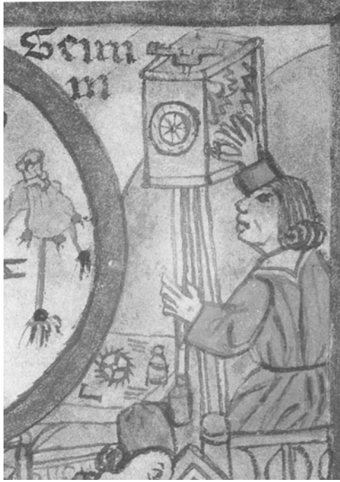
Plate 1 A clockmaker at work, c. 1450–75. From part of an astrological treatise showing occupations involved in astronomy and prognostication, the drawing shows a part-disassembled domestic wall clock, with its foliot bar projecting above the clock case, weights and cords suspended beneath it, and a gear wheel, parts, and tools on a bench or shelf. Though turret and domestic clocks differed considerably in scale their mechanisms could be very similar in other respects. Reproduced by permission of The Bodleian Library, University of Oxford, MS. Rawl. D1220, fol. 32.
