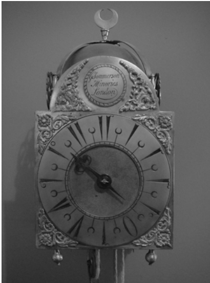
Plate 6 A London clock for export markets, c.1700. By the late-seventeenth century clocks were being exported from London to many parts of the world. This example came from an established maker in the City, with a sideline in clocks for the Turkish market. Though with some features directed to that context, on the dial and on top of the clock, this is a basic single-handed design of pre-pendulum type, but benefiting from larger scale production, and more specialized production of components. Photograph courtesy of the private collection of Mark Taylor.
